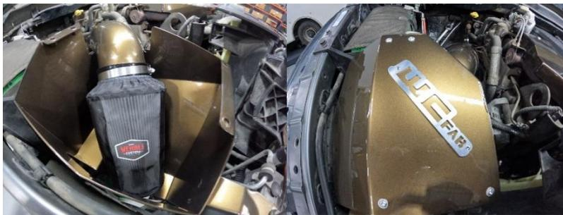
11. Tighten intake tube clamp on turbo side, then slide ccv hose onto pipe coming from the engine and tighten clamp.
