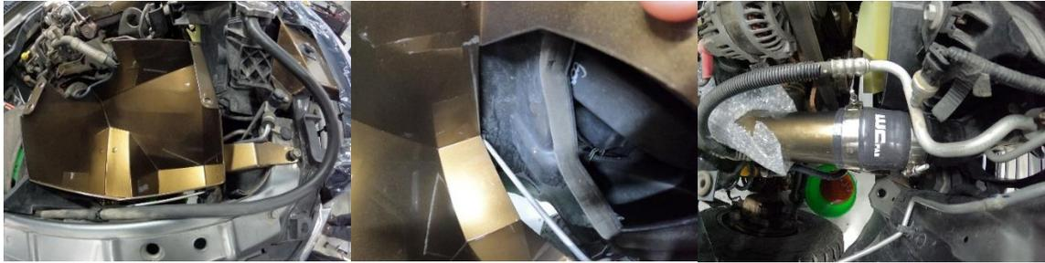
9. Using some Assemblee Goo or similar product, install intake pipe into boot at turbo inlet and position it so tube lays into box and has proper fitment into turbo and box.
