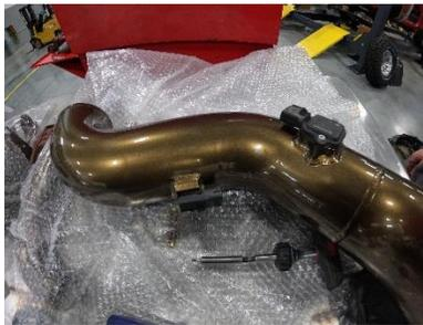
6. Install CCV hose onto new intake pipe and tighten clamp.
