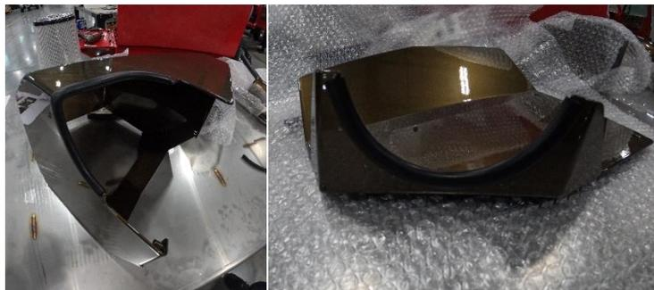
8. Install airbox into place and verify fitment of air box. Check intercooler clamp to box clearance as well as high-pressure ac line on the front corner of the box near fender.
