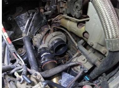
5. Remove sensors from original intake tube and install them into new intake pipe.
