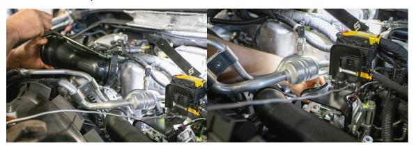
7. Install studs into the turbo housing by hand until they bottom out.
