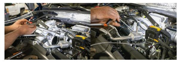
6. Remove factory intake horn.
