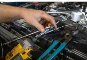
9. A small amount of grease is used to hold nut in socket during assembly.
