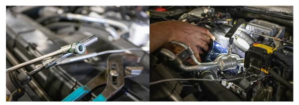
10. Torque to factory spec (25 nm/18 ft. lbs). There are two nuts holding the intake horn to the turbo housing.
