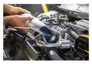
8. Install the box back onto the pipe and tighten the screws to hold the airbox lid on. Tighten all clamps evenly. Plug the MAF sensor back in.
