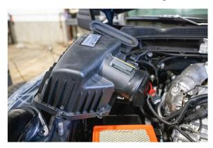
4. Install the boot and clamps onto the intake horn. Do not tighten yet.
