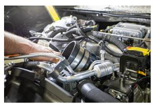
5. Install the boot and clamp to the airbox. Install to airbox outside of the truck on the bench. Use the socket to assist in pushing the nut onto the stud. This will be tight for the first install and is normal, once it has been used it will be able to easily install and remove clamp at air box for normal service and filter inspection.
