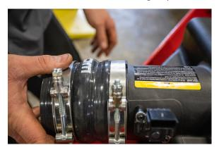
7. Loosely install the pipe into the boots. Do not tighten any clamps to allow proper alignment.
