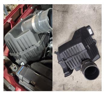
7. Remove the 3 rubber grommets from the factory box. There are 2 towards the back and 1 where the nut was in the previous step.
