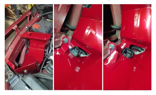
10. Reinstall the 10mm nut to hold the new intake box in.
