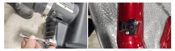
14. Install the intake tube to the horn with the 4" boot and clamps.
