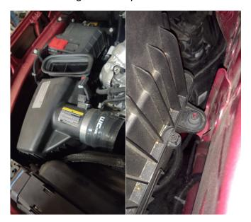
6. Remove the factory intake box by lifting it up. There are two rubber grommets at the back of the intake that pop out.
