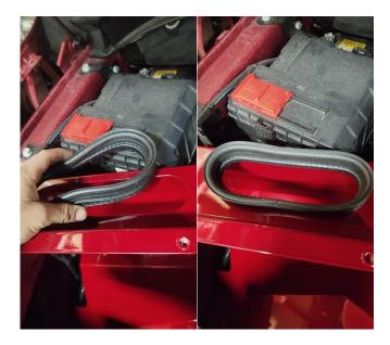
12. You will need to cut the smaller weather stripping evenly in half. Take one half and install it onto the lower half of the box. Push firmly over the edge of the box and trim any excess once you reach the end of the cut out gasket area. Do the same on the other half of the intake box.
