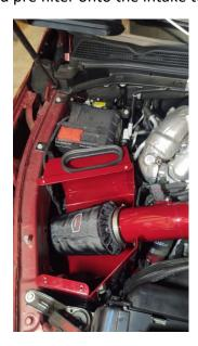
17. Tighten the clamps holding the pipe to the horn after clocking to the correct position.
