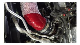
18. Install the upper half of the intake box using the 4 supplied bolts.
