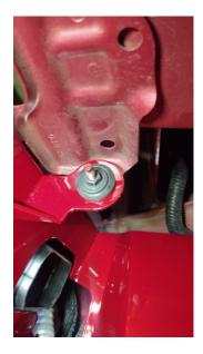
11. Install the large weather stripping into the top hole that provides a seal between the hood and the intake box.
