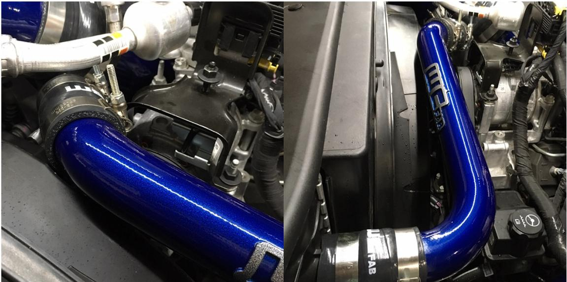
8. Tighten the clamps, refill the cooling system and start the truck allowing it to get up to normal operating temperature.
