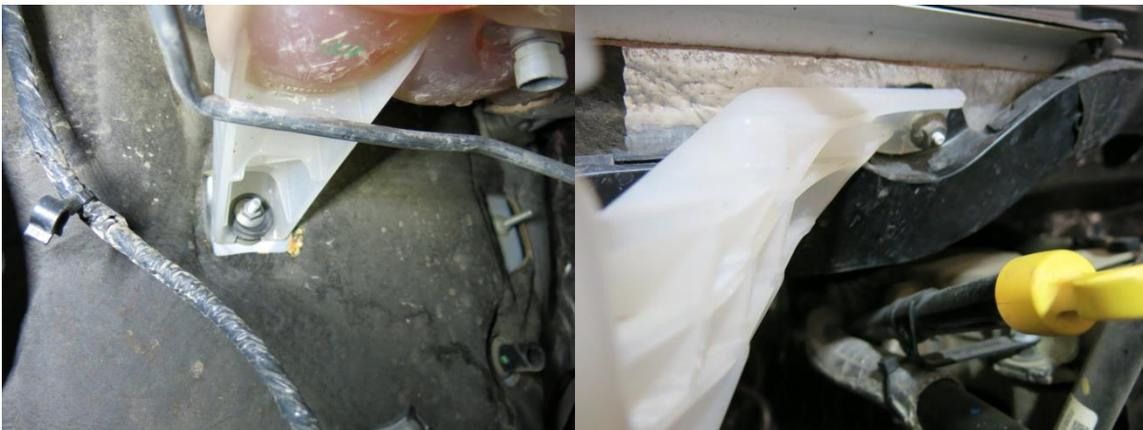
10. Remove the coolant tank.
