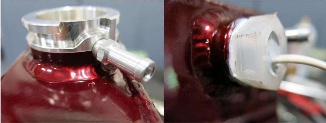
12. Install new tank. Use lower existing stud & new 6mm bolt in threaded hole in fender.
