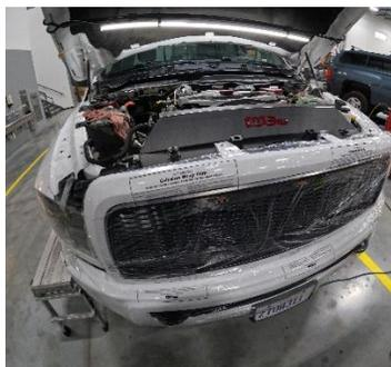
6. Tighten the 6 bolts by hand to the grille and radiator shroud.
