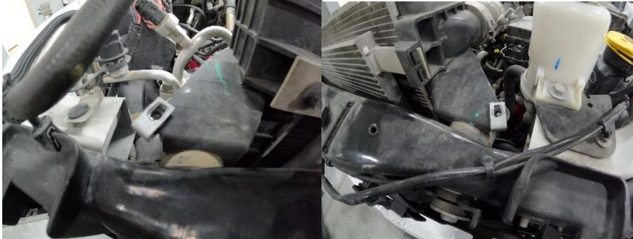
4. Hold the cover in position and start the two outer bolts into the J nuts previously installed. (DO NOT TIGHTEN).
