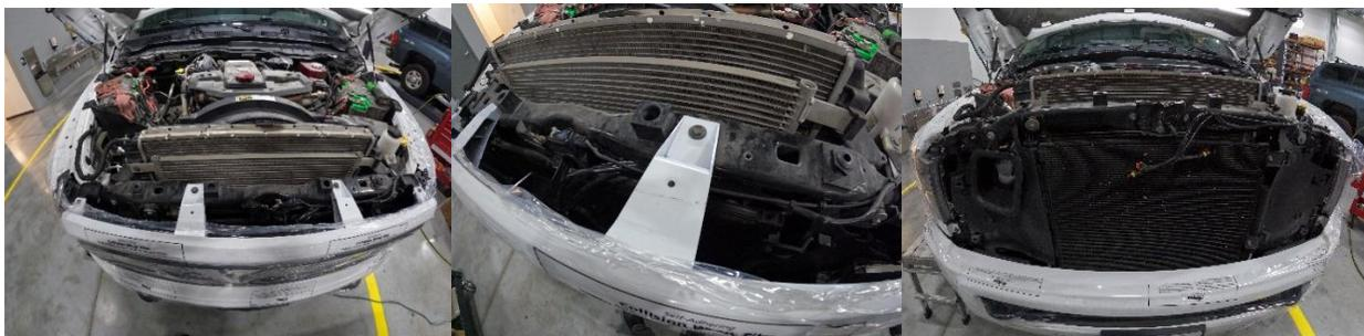
3. Install the two J nuts in the locations shown at the outer tabs on the radiator.
