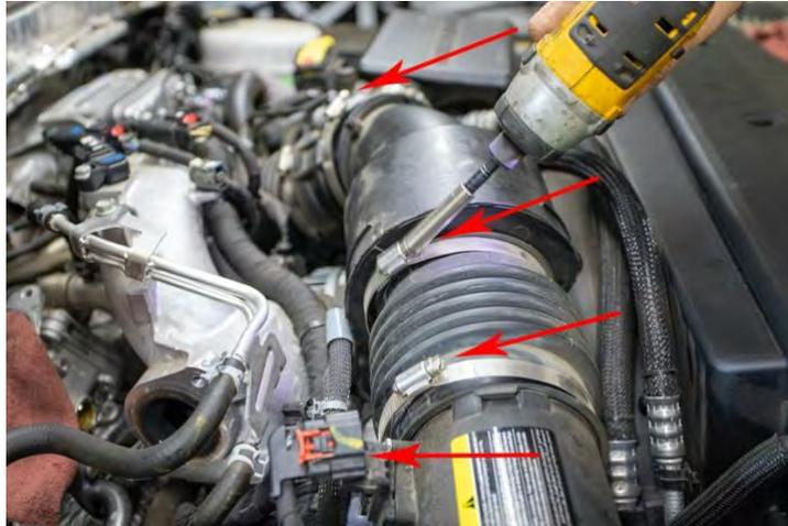
5. Unplug MAF Sensor and disconnect intake pipe
