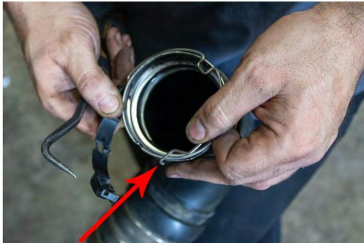
15. Remove clip ring from lower OEM Intercooler pipe connection using a pick or flat blade screwdriver.
