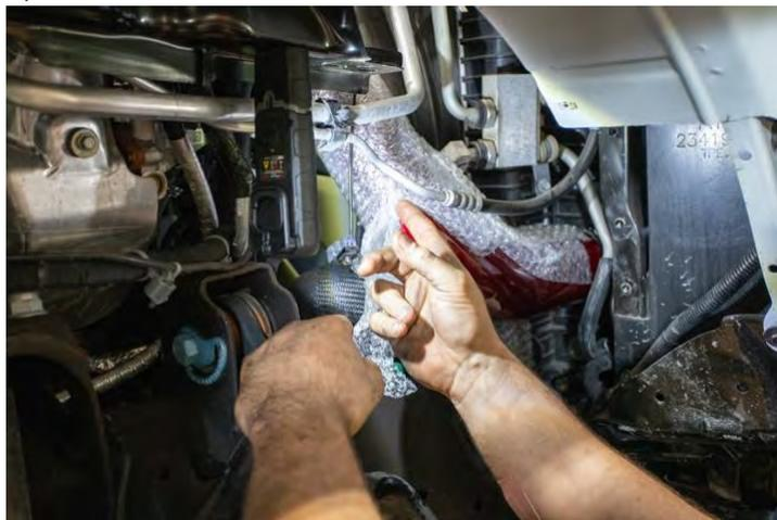
25. Remove bubble wrap from piping and clean any fingerprints with damp microfiber cloth.
