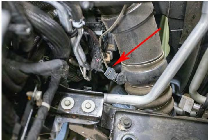
9. Unplug Charge Air Temp Sensor on Intercooler Pipe.
