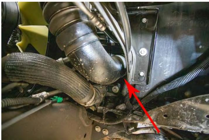
11. Access and locate clip ring at lower intercooler pipe connection through wheel well.
