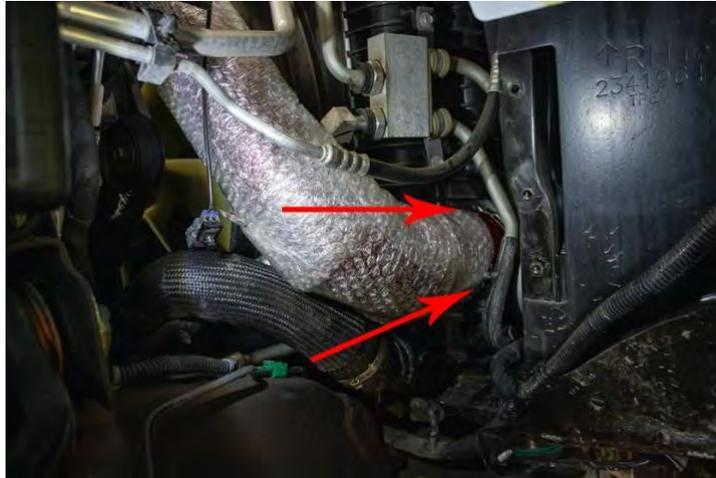
23. Move to lower assembly and fully seat the clip ring so that it is engaged / down all the way. Adjust pipe at upper connection as necessary once lower clip is seated. Lower airbox brackets have been removed for illustration purposes. It is not necessary for installation but can provide additional workspace if needed for accessing the clip assembly.
