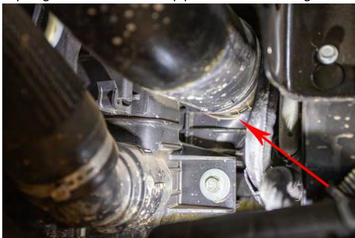
12. Using a pick or flat blade screwdriver, remove clip at lower intercooler pipe connection and pop pipe off of intercooler.
