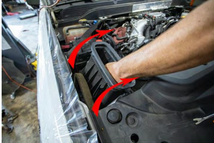
8. Separate Lid from Airbox. Grab Lower Airbox and pull up firmly to unseat the lower airbox from the inner fender.
