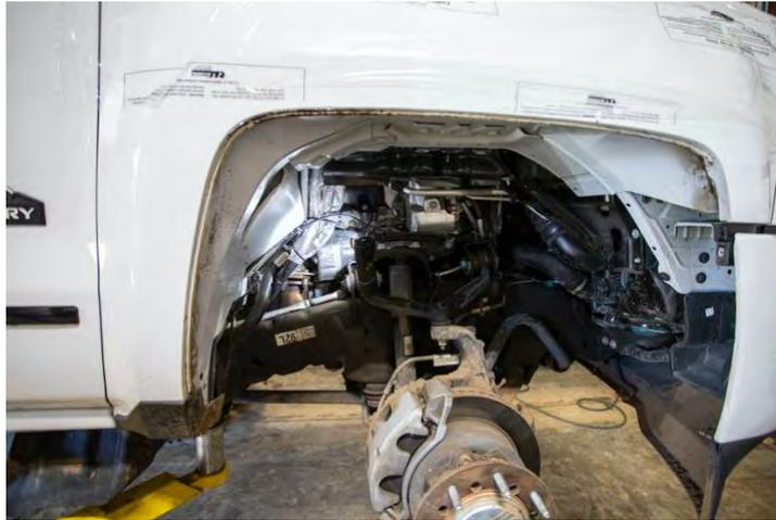
4. Remove the passenger side wheel/tire and inner fender liner.
