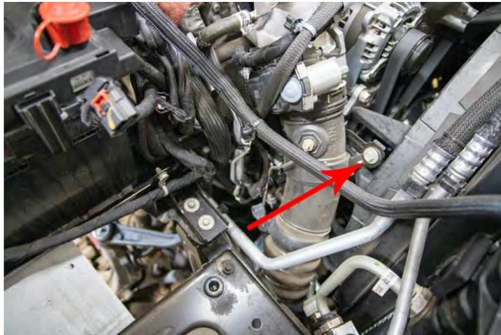
10. Remove Bracket Bolts from the intercooler pipe.
