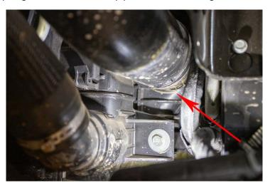
10. Using a pick or flat blade screwdriver, remove clip at lower intercooler pipe connection and pop pipe off of intercooler.
