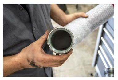
13. Install new clip ring to the new intercooler pipe assembly. NOTE: Pay close attention to orientation of clip ring on the new pipe as it will only properly engage the pipe and intercooler assembly one way. One groove in the pipe is smaller than the other two. Reference image above to make sure your ring position matches the mounting shown.
