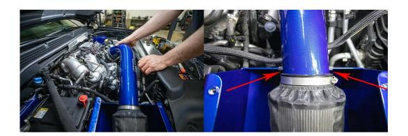
16. Install Intake pipe with filter assembly into hump boot at horn and adjust pipe placement and filter depth as necessary to allow a gap as shown in image above between filter and air box seal.
