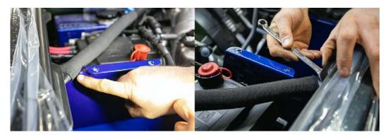
8. Note: Build tolerances vary from truck to truck. Many trucks will require no adjustments for your air box installation. However, on some trucks, the fender brace may contact the air box as shown in this image. To correct this, first loosen the brace at the fender using a 13mm wrench.
