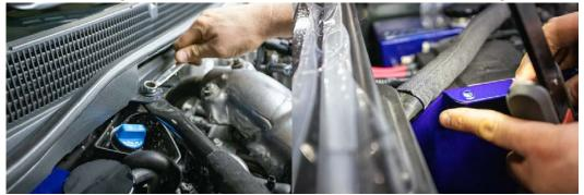
9. Next loosen the connection at the firewall and slide brace away from air box to achieve clearance (as shown above). Re-tighten brace once proper fitment is achieved.
