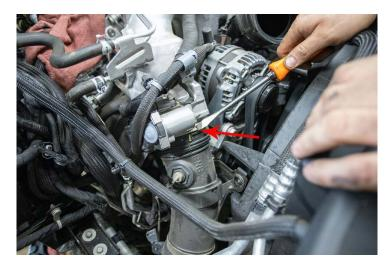
11. Turn lock ring clockwise to remove top connection to engine and slide pipe off of intake flange.
