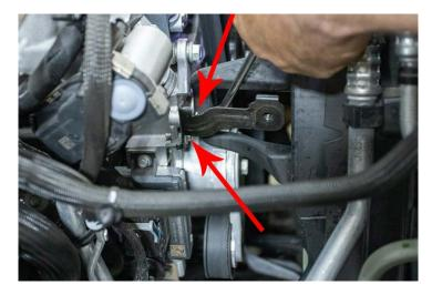
16. Remove OEM Intercooler support bracket from engine as it is no longer required.
