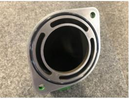
6. After boost testing is complete, the new turbo intake horn can be installed. Install O-ring into the groove of your new intake horn using a very small amount of grease to hold in place if needed on
