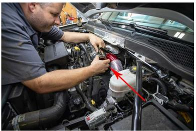
11. Install reducer boot at turbo
