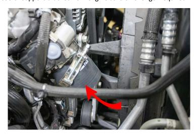
17. Install top boot and clamps onto the engine intake side and leave loose.
