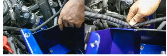
10. Install supplied pipe seal on lower air box and trim to fit saving excess for use on the lid in Step 19. Next install coolant line retainer clip into pre-drilled hole in your new air box assembly.
