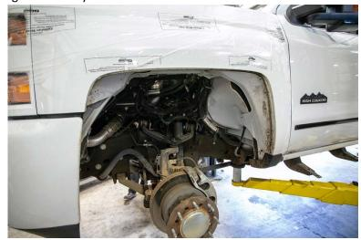
4. Remove the driver side wheel/tire and inner fender liner.
