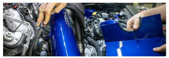
18. Reinstall MAF sensor connector and install remaining pipe seal on upper air box lid trimming excess. Check pre-filter placement & filter clamp is tightened before proceeding to next step.
