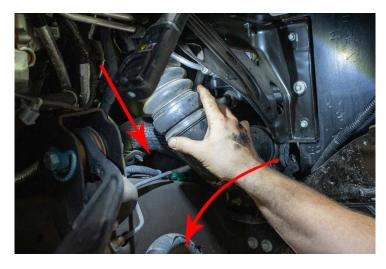
12. Remove pipe by passing it out carefully through passenger wheel well.
