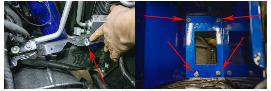
7. Install supplied nutsert, reinstall lower air box and install saved OEM 10mm fasteners from Step 2 working clockwise from rearmost engine side first, completing fender side last. Adjust box alignment as necessary while completing this process.
