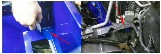
6. Adjust air box position, then use a paint pen to mark location on the lower brace that needs to be drilled for the included nutsert. Remove lower air box and drill marked hole as shown. Verify that nothing is under the location being drilled before making the required hole in the bracket.
