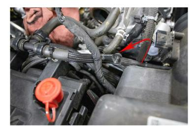
5. Remove Wire Harness Clip and tuck safely out of the way.
