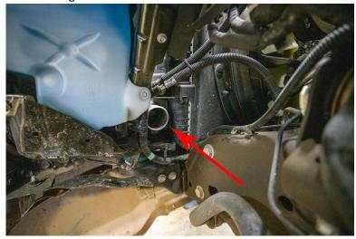
8. Clean off turbo and intercooler connection points with brake cleaner if needed.
