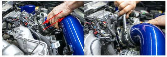
17. Adjust pipe depth at intake horn boot to allow proper seating of clamps to the pipe bead roll seal and then tighten assembly. Do not push pipe in past the point when you feel bead roll enter opening in hump boot.
