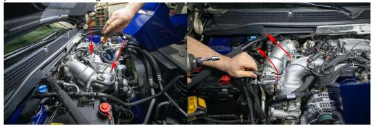
3. Unbolt retaining tabs (2x 10mm bolts) shown. Shift coolant hardline gently out of the way to provide clearance for new air box installation preventing scratches to the powder coat finish.
