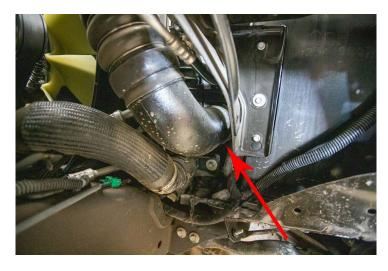
9. Access and locate clip ring at lower intercooler pipe connection through wheel well.
