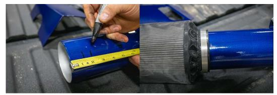
12. Using a tape measure and a marker, place small mark at 2" from filter end of your new intake pipe to help set mounting depth. Install filter onto pipe leaving mark exposed. **Improper filter depth can cause air restriction on your new intake.** Do not tighten filter clamp at this time.
