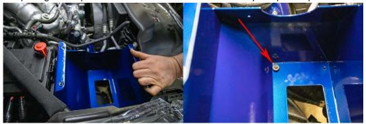
5. With lower air box in place, loosely install rear OEM bolt indicated to locate assembly.
