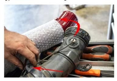
14. Swap charge air temp sensor from OEM intercooler pipe to your new 3.5" intercooler pipe using a pry tool to remove wire harness clip and a 14 mm wrench. Liquid Teflon thread sealant is recommended on the sensor during re-installation for a leak free seal.
