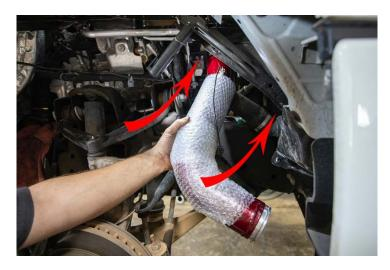
18. Install new intercooler pipe upwards carefully through passenger side wheel opening paying attention not to damage charge air temp sensor.
