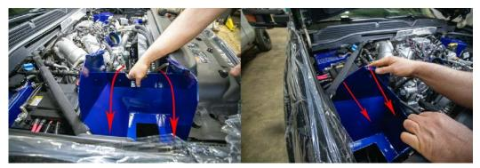
4. Install lower air box as shown. It may be necessary to gently bend rear wall of the box to clear the fender brace if you choose to leave in place as shown. **This box goes in without force.**
