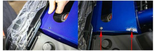
20. Adjust lid to align front air box mounting holes and loosely install supplied fasteners to locatethe assembly.
