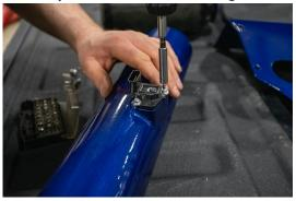
13. Remove MAF sensor from OEM air intake and reinstall on your new air intake pipe using supplied hardware and maintaining correct orientation. **The Original MAF sensor screws will not work.** Do not try to install them on your new pipe.
