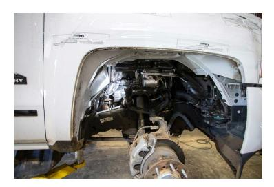
2. Remove the passenger side wheel/tire and inner fender liner.
