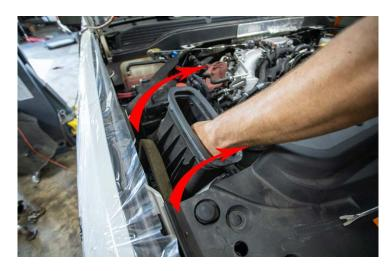
6. Separate Lid from Airbox. Grab Lower Airbox and pull up firmly to unseat the lower airbox from the inner fender.
