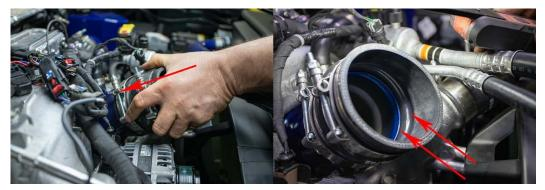
14. Install hump boot and clamps onto intake horn paying close attention to match alignment of horn lip to hump shown as indicated in image above.
