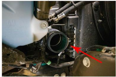
9. Install straight boot at lower intercooler pipe connection
