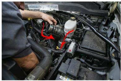
7. Remove pipe from truck using whatever means is easiest for you. We typically recommend taking the pipe out and down through the wheel well area.
