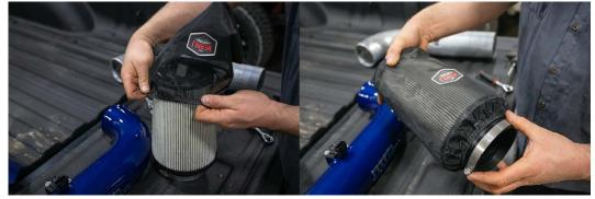
11. Install pre-filter cover and clamp on air filter as shown.
