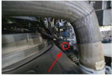
6. Remove clamp at intercooler on driver side bottom.
