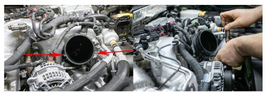
2. To remove OEM intake horn, locate and remove bolts shown in images above. This can be done using a long ¼" extension and 13mm swivel socket. There is no reason to remove any other items for access.
