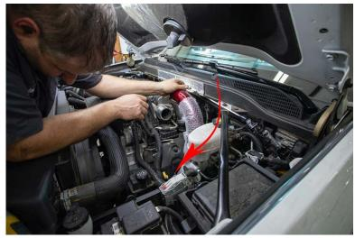
10. Install pipe from top side of engine compartment paying attention to match orientation of original pipe design.
