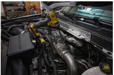
5. Remove clamp at turbo outlet.
