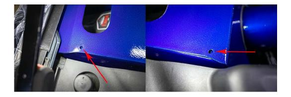
19. NOTE: When installing upper lid of your intake air box some amount of misalignment may occurbetween the box and lid as shown in the images above. Follow steps below to properly adjust alignment and complete your installation. Do not force screws into holes.
