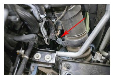
7. Unplug Charge Air Temp Sensor on Intercooler Pipe.
