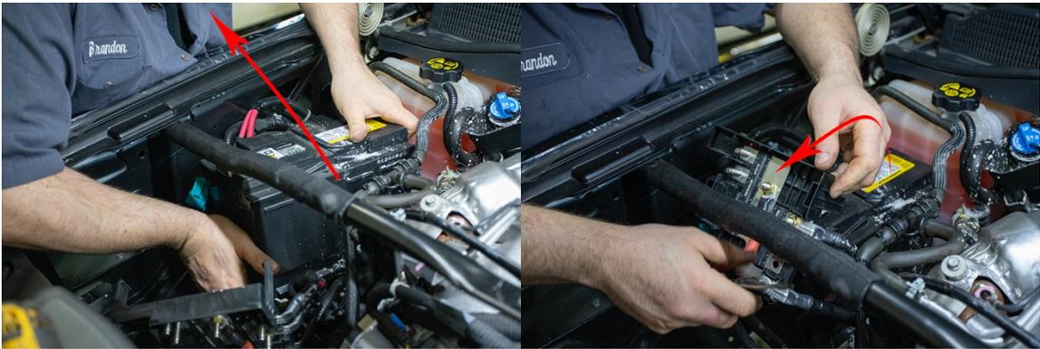
5. Now, remove the hoses from the coolant tank. They will have a spring clip holding them on. If they are stuck to the tank, you can use a hose removal tool with caution to not damage your hose. Remove the level sensor prior to pulling the tank.
