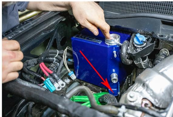
9. Reconnect the factory hoses onto tank. At this time, you can install the overflow hose that came with your new tank. Route so that this is not laying on or near the engine or the exhaust manifold.
