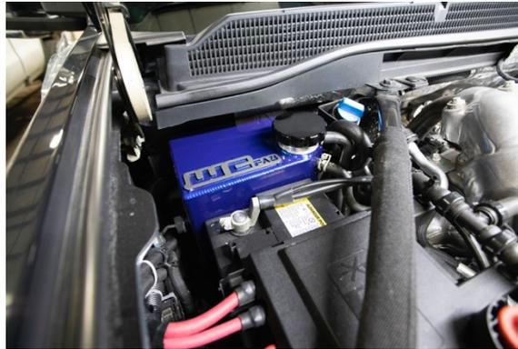
1. Disconnect both batteries. Ensure you have no power to the truck. You will need to drain some coolant from the system or pinch off hoses to minimize coolant loss.
