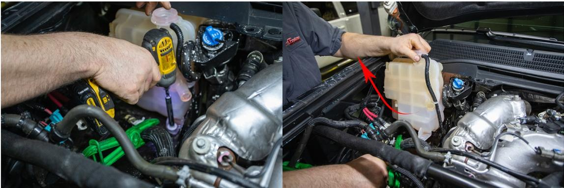
7. Install the new level sensor into your new tank. These are pipe threads and require sealant. We recommend using a liquid pipe thread sealant. Tighten the sensor up and make sure to have the arrows on the sensor facing up. You will also install the overflow nipple just under the cap. **NOTE: White hex sensor needs arrow pointing up, black round sensor needs arrow pointing down.**
