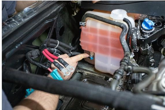
6. Remove the one 10 mm bolt at the lower front corner closest to the engine and slide the tank to the front of the truck. It will release from the two rear mounting points.
