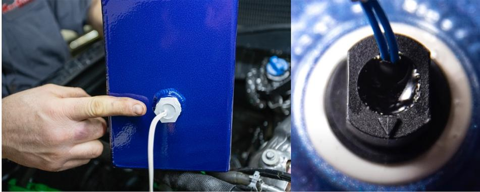
8. Plug in the level sensor into the truck side harness and install the tank making sure you get the rear mounting points aligned and slide back into position. Now, you can install the 10 mm mounting bolt.
