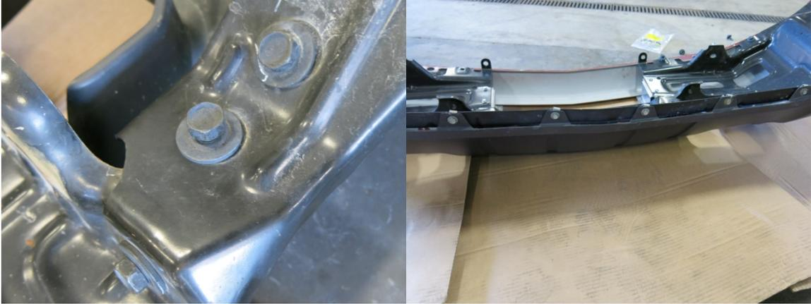
6. Remove both bumper support brackets and fog lights from each side of the bumper. There are five 15 mm bolts on each side.
