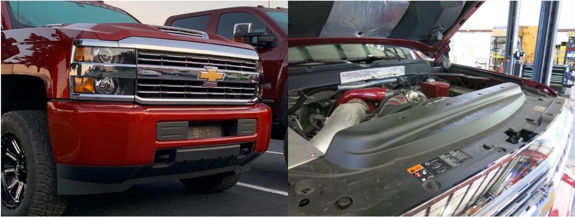
2. Remove plastic radiator cover under hood by removing twelve plastic pop rivets to reveal radiator stack.
