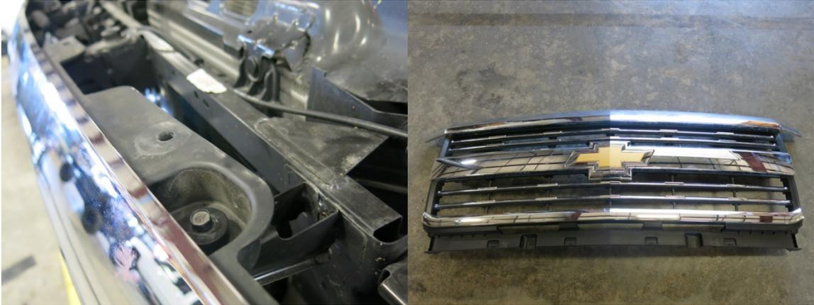
4. Remove front bumper. There are four bolts in the center and one on each end in front of the tires. Disconnect the wiring harness underneath the bumper towards the passenger side. The Bumper harness stays on the bumper for removal. Unplug fog lights if equipped. Lay bumper face down on cardboard or towel.
