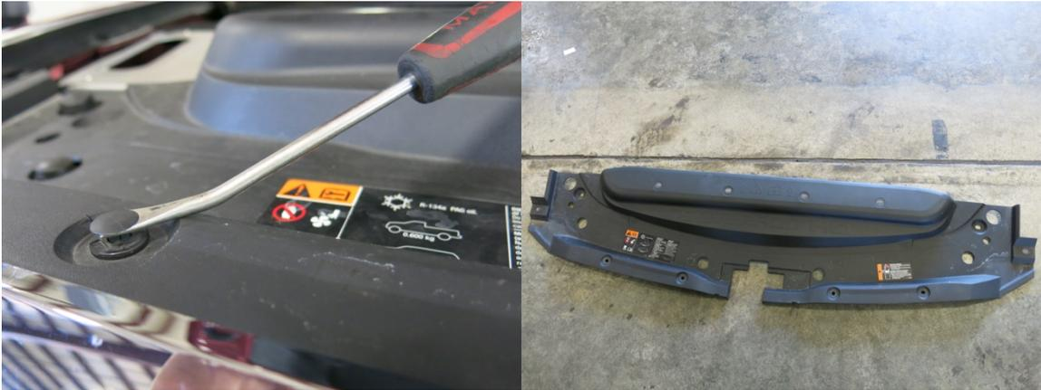
3. Remove grille. There are four bolts on top and push disconnects.
