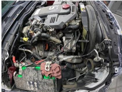
4. Loosen intercooler pipe clamp at turbo outlet.
