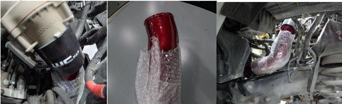
19. Tighten all clamps for driver side pipe at top and bottom connections.
