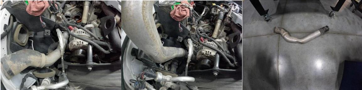
6. Clean connection points at intercooler and turbo outlet for new boots.
