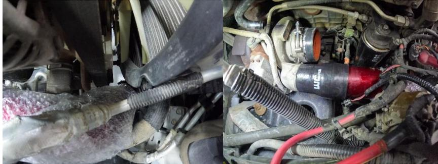
11. Center the pipe and boots to allow for correct clamp installation. Make sure the clamp sits past the beadroll to avoid blowing off while driving. Tighten all the remaining clamps that have not been previously tightened.
