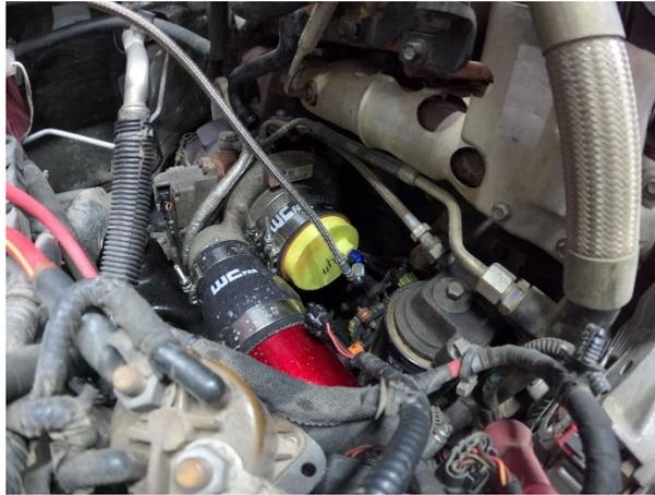
21. Install shield at intake air valve, inner fender, wheel and tire. Reinstall the air box and any connectors removed for install. Connect battery terminals and start engine to verify the engine light does not come on. If you do get a engine light, check that the sensors have all been successfully connected and are functioning properly.
