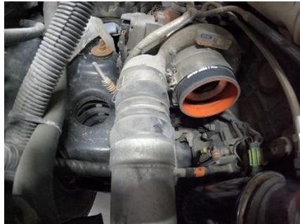
5. Remove intercooler pipe clamp at intercooler and remove stock pipe from truck. You may need to use a hook tool to aid removal of old boots at the connection points. Removing the pipe from the truck can be done by rotating it while pushing back towards firewall.
