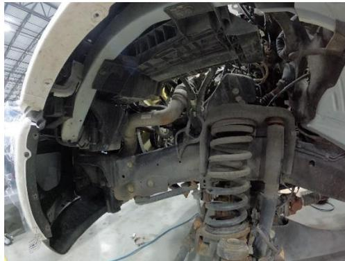
15. Remove clamp at the driver side intercooler connection working through the inner fender area. Remove pipe from the truck.
