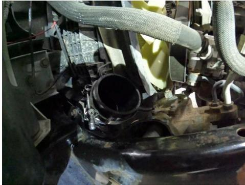
17. Install boot at intake air valve, do not install clamps yet at this connection.
