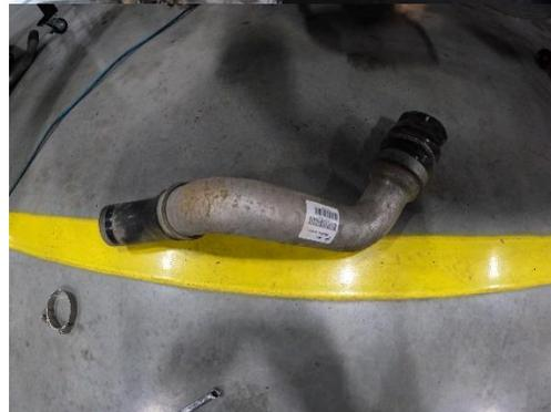
16. Clean both intercooler connection points at the intake air valve and the intercooler. Install the new boot at the intercooler outlet and tighten the clamp at the intercooler connection only.
