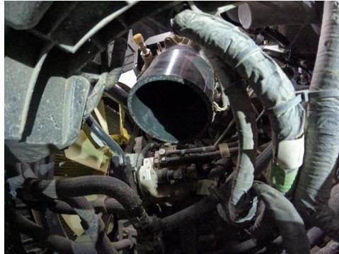
18. Use Dr. Tranny's Assemblee GOO or similar product on both ends of intercooler pipe to aid install of pipe into boot on intercooler. Make sure clamps are on pipe so they can be slid up to the boot once it is in place.
