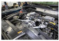
2. Remove valve cover breather hose from intake horn by twisting and pulling up at the same time. Usually, the metal clamp can stay in place and you can slide directly on to the new intake horn.
