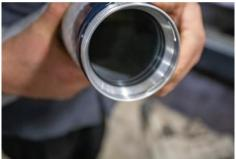
14. Install the adapter onto the engine side connection. You may now use a small amount of assembly lube such as Trans-Jel or Dr. Tranny's assembly goo. You may use a small amount of dielectric grease if you are not able to locate suggested items. Avoid using petroleum or other synthetic that may damage the oring seals.
