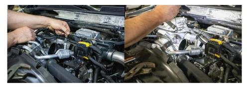
4. Remove two 13 mm head bolts holding the turbo inlet horn to turbo using a long extension and swivel socket (1/4" drive).
