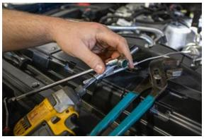
8. A small amount of grease is used to hold nut in socket during assembly.
