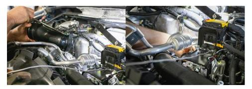
**Note**: While the intake horn is removed, boost testing is recommended after installation and service of the intercooler piping. Boost testing (Boost Tester Kit Sold Separately Part# 13U7H001) is always recommended whenever intercooler pipes have been serviced or boots and clamps have been moved.
