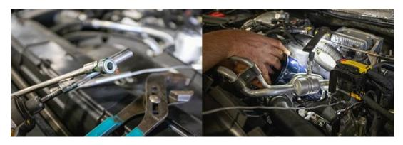
9. Torque to factory spec (25 nm/18 ft. lbs). There are two nuts holding the intake horn to the turbo housing.
