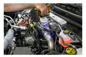
4. Remove the clamp at the intercooler connection utilizing an 11mm socket and extensions as shown in the image above.
