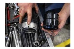
12. Swap charge air temp sensor from OEM intercooler pipe to your new 3.5" intercooler pipe using a 14 mm wrench. A very small amount of liquid Teflon thread sealant is recommended on the sensor during re-installation for a leak free seal.
