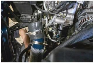
18. Using the supplied boot and clamps, apply a thin layer of assembly goo into both ends of the boot. You may hold it in between the intercooler pipe and adapter at the engine as pictured.
