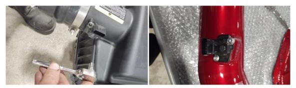
8. Install the intake tube to the horn with the 4" boot and clamps.
