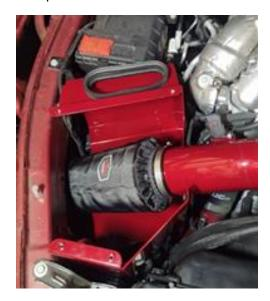
11. Tighten the clamps holding the pipe to the horn after clocking to the correct position.
