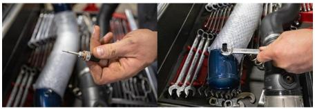
13. Install o rings into the connection points for the passenger intercooler pipe: two at the engine and two at the intercooler. It is best to install them dry. \*\*\* DO NOT USE ANY LUBRICANT AT THIS TIME \*\*\* Install the two larger o rings into the adapter that goes onto the engine side connection. Install the two smaller o rings into the lower end of the intercooler pipe where it attaches on to the intercooler. When installed correctly, the o rings should be uniform and even.
