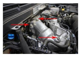
12. Remove EGR upper mounting bolts. There are two more bolts not visible in this picture where this pipe connects to the SCR under the cowl which also need to be taken out in order for the pipe to be completely free of the engine.
