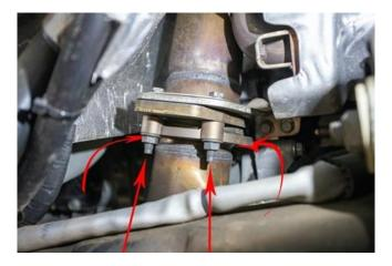
33. Reinstall rear heat shield on passenger side exhaust manifold (3x 10mm bolts)
