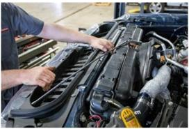
5. Remove the pipe from the truck by lifting and rotating it out from the top of the engine bay.
