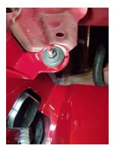
5. Install the large weather stripping into the top hole that provides a seal between the hood and the intake box.
