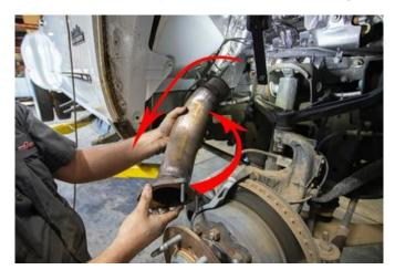
21. Reinstall downpipe temperature sensor taken from stock part.
