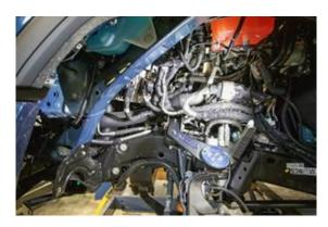
2. Disconnect the ecm wiring harness and move out of the way with bungee cords to allow access during removal and install.
