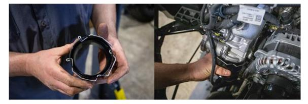
15. Apply a thin layer of Assembly Goo to the orings at the lower connection where you previously installed the two orings into the pipe and a very thin layer onto the intercooler where the pipe will be installed.
