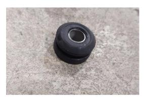
2. Transfer the grommets to the proper locations. The two pictured should go into the holes in the truck.
