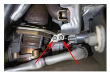
6. Remove upper down pipe support bracket which connects to the back of the cylinder head.
