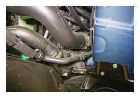
7. Using a pick or flat blade screwdriver, remove the clip at lower intercooler pipe connection and remove from the intercooler.
