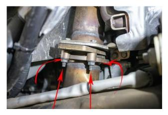
5. Remove lower down pipe support bracket which connects to engine block.
