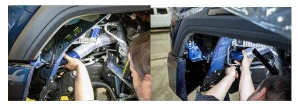
10. Install the upper part of the pipe into the boot connection at the turbo and tighten the clamps at the turbo and intercooler connections. Make sure the pipe is properly aligned and clamps are properly positioned on the boots to avoid blowing the boot off.
