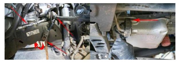
32. Reinstall lower v-band clamp to connect exhaust system to bottom of downpipe.
