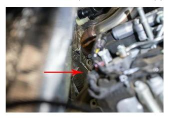
17. Remove top bracket from down pipe. There are no good sight lines to the bolts holding this part in but the items removed in the steps above will allow enough room for you to access this bracket through the passenger wheel opening and from the engine bay above.
