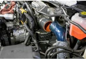
9. Install the pipe into the boot at the intercooler connection, making sure the clamp and boot are past the bead roll on the pipe to avoid blowing the boot off.
