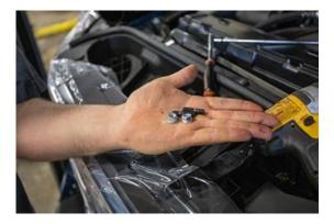
7. Now, install the intake horn onto the studs. A small amount of grease or assembly gel can be used to keep the o-ring in place.
