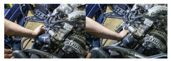
20. Now loosely install the clamps and align boot with pipe for proper placement. This should be even on both ends and allow enough room to clamp properly.
