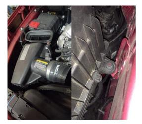
4. Remove the factory intake box by lifting it up. There are two rubber grommets at the back of the intake that pop out.
