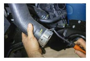
8. Remove clip at engine side of passenger intercooler pipe.
