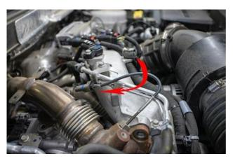
14. Remove EGR Pipe and set aside being careful not to damage riveted on gaskets which will be needed for reinstallation later.
