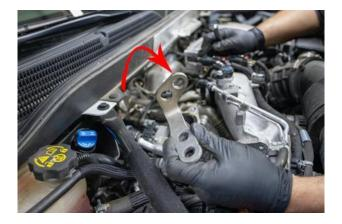
26. Reinstall lower downpipe bracket.
