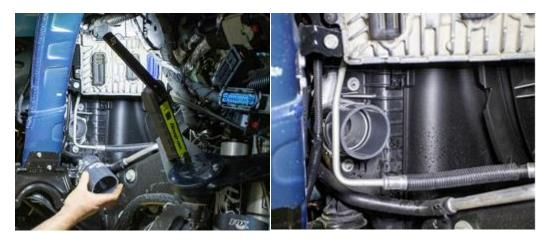
7. Install the reducer boot and clamps at the turbo connection point. Only tighten the clamp at the turbo outlet.
