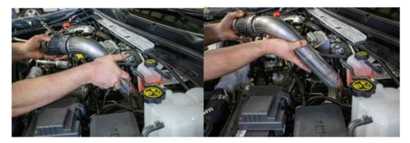
6. Make sure the lower intercooler pipe connection is clean and install the straight boot/clamps. Only tighten the clamp on the intercooler connection, the other will remain loose until the pipe is properly positioned.
