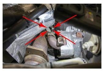
7. Remove front rubber exhaust hangar from exhaust system near transmission. This step allows the exhaust to drop to allow room for down pipe removal.
