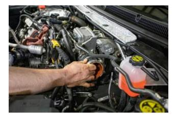
8. Install the new driver side pipe up through the wheel well. Trans assembly lube can be used to ease assembly of the pipe into the silicone boot connections. We specifically use the green Dr Tranny's Assemblee Goo transmission assembly lube during install.
