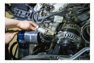
19. Rotate the intercooler pipe to the engine as seen and it will slide right into place.
