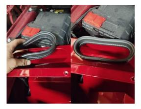
6. You will need to cut the smaller weather stripping evenly in half. Take one half and install it onto the lower half of the box. Push firmly over the edge of the box and trim any excess once you reach the end of the cut out gasket area. Do the same on the other half of the intake box.
