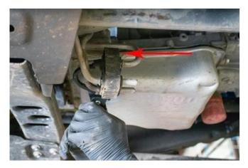
8. Ratchet strap placed around front of exhaust pipe near joint and wrapped under frame rail, and clipped at upper control arm may help provide leverage if needed to draw exhaust down and out of the way. Note: This image is for illustration purposes and was taken after the downpipe had already been removed.
