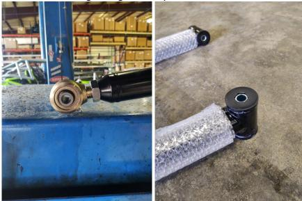
4. Install the bushing end of the traction bar into the U-bolt bracket. Use the longer set of bolts with two washers and 1 nylock nut each. Install the bolt from the center of truck out so that the threaded end will be closest to tire.
