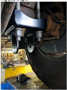
3. Install the bushings and heims into the traction bar. Use grease or brake lube to help bushings slide while being installed. Use a small amount of anti-seize on the threads of the heims. Install the heim into the traction bar as seen in photo. Leave the bubble wrap on bars to avoid scratching during assembly.
