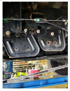
7. Once cooled and painted, reinstall traction bars. Grease heim joint fittings and tighten jam nut and bolts. Remove the protective bubble wrap.
