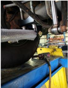
5. Install the frame side bracket onto the heim using the shorter set of bolts. Install the bolt from the outside of the truck inward for a better appearance.
