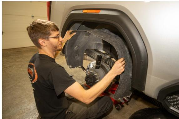
5. Disengage most of the fender clips exposing the light.
