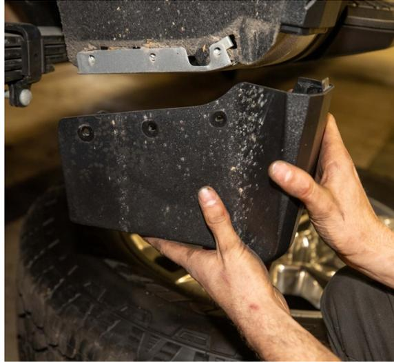
4. Remove the fender liner, which consists of two 10 mm plastic nuts, one screw nut on top and all T-15 screws.
