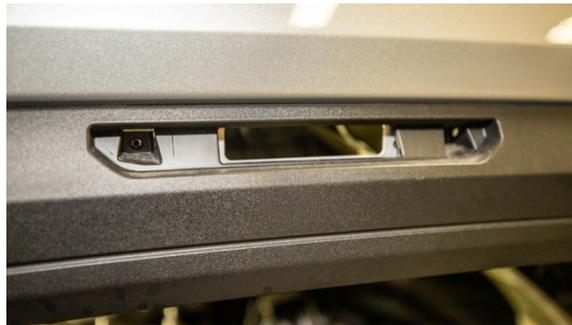
7. Install the WC Fab delete into the truck and use supplied hardware (**not** the factory T-20).
