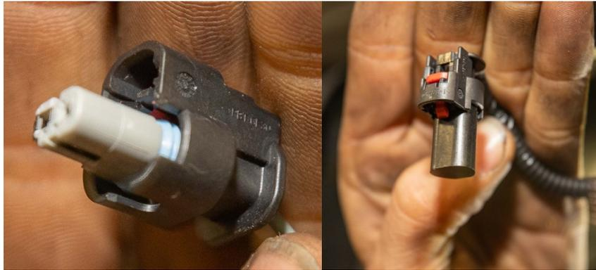
4. Install isolating plug to vehicle side wire harness. You should hear a click when installed.
