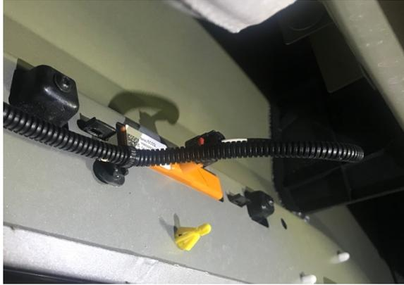
9. Remove the light (two T-20 screws).
