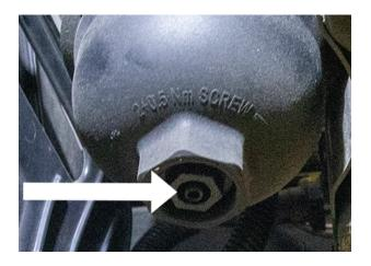
4. With the pan or container still under the filter, disconnect both quick disconnect fittings from the OEM filter base.
