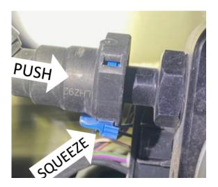
To unseat the white locking tab, FIRST release the locking tab on either side of the connector body. SECOND, gently lift or pry it upward to release.
