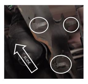
6. Remove the 3 cap screws securing the fuel heater to the OEM filter base using a T30 torx bit.
