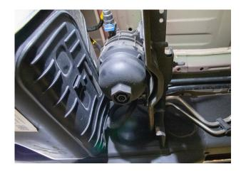
Place a pan or a container below the OEM fuel filter.
