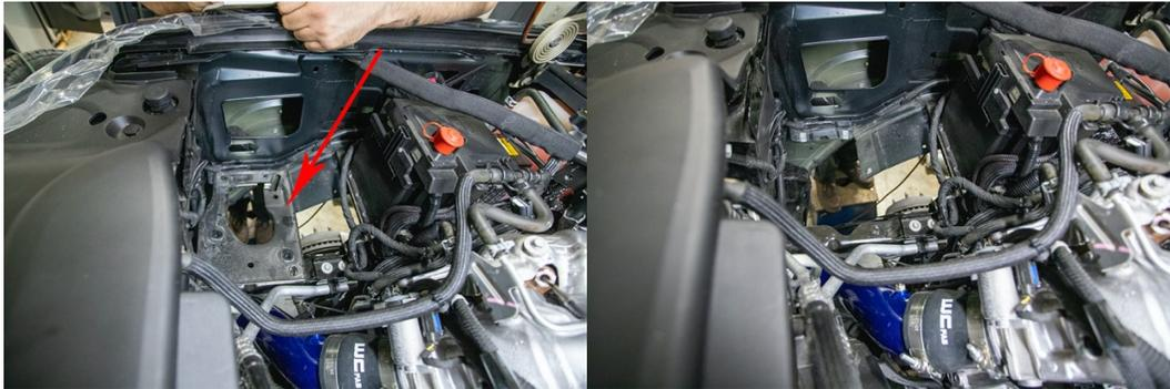
7. Remove 10mm bolts and set aside for later re-use. Remove and discard lower air box mounting plate which will no longer be used.
