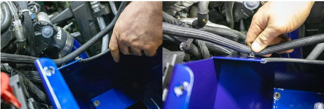
15. Install supplied pipe seal on lower air box and trim to fit saving excess for use on the lid in Step 26. Next install coolant line retainer clip into pre-drilled hole in your new air box assembly.
