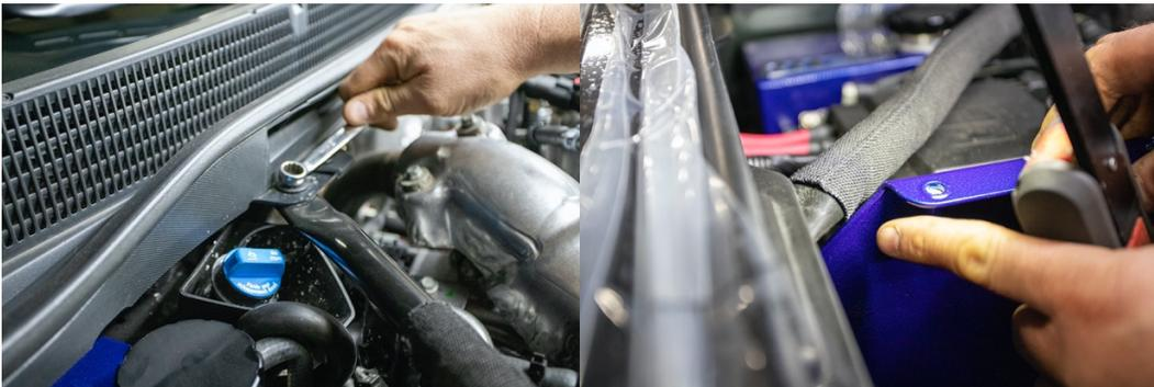
14. Next loosen the connection at the firewall and slide brace away from air box to achieve clearance (as shown above). Re-tighten brace once proper fitment is achieved.
