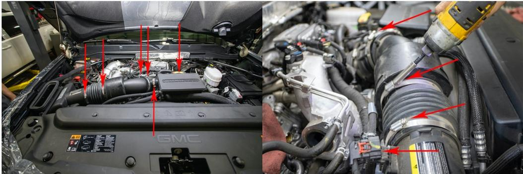
4. Unplug MAF Sensor and disconnect intake pipe by disconnecting clamps and fasteners at the points indicated in the images above.
