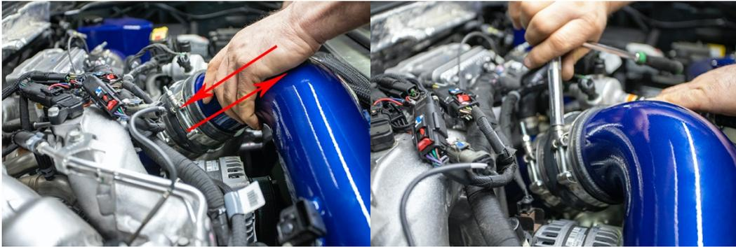
24. Adjust pipe depth at intake horn boot to allow proper seating of clamps to the pipe bead roll seal and then tighten assembly. Do not push pipe in past the point when you feel bead roll enter opening in hump boot.
