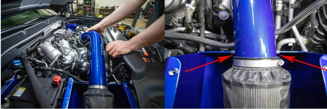
23. Install Intake pipe with filter assembly into hump boot at horn and adjust pipe placement and filter depth as necessary to allow a gap as shown in image above between filter and air box seal.
