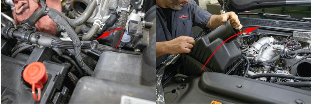
6. Remove coolant line clip and tuck safely out of the way. Next, remove OEM air box. Grab and pull up firmly to unseat from the inner fender.
