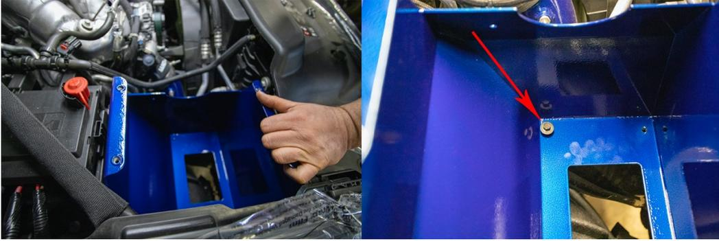
10. With lower air box in place, loosely install rear OEM bolt indicated to locate assembly.
