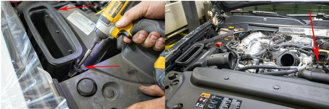
5. Unbolt Airbox and Resonator. Remove resonator and intake piping.
