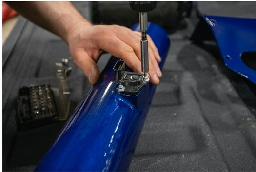
18. Remove MAF sensor from OEM air intake and reinstall on your new air intake pipe using supplied hardware and maintaining correct orientation. **The OEM MAF sensor screws will not work.** Do not try to install them on your new pipe.
