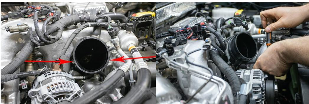
19. To remove OEM intake horn, locate and remove bolts shown in images above. This can be done using a long  $\frac{1}{4}$ " extension and 13mm swivel socket. There is no reason to remove any other items for access.
