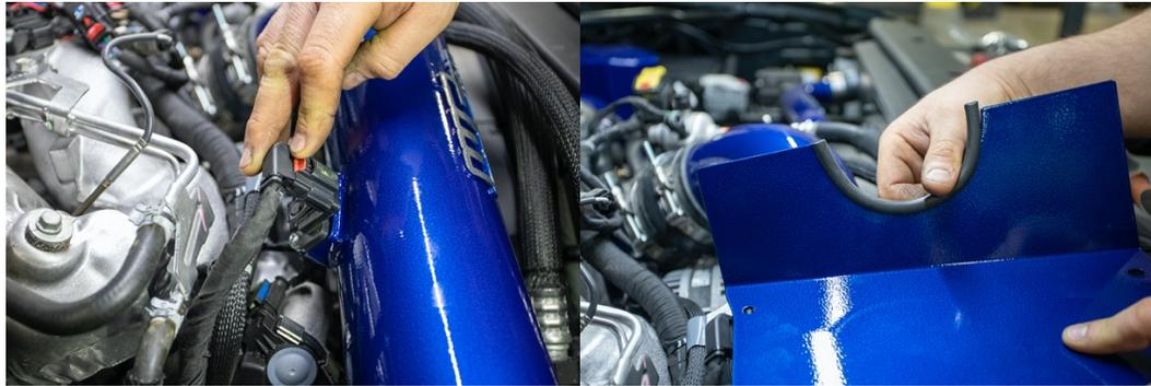
25. Reinstall MAF sensor connector and install remaining pipe seal on upper air box lid trimming excess. Check pre-filter placement & filter clamp is tightened before proceeding to next step.
