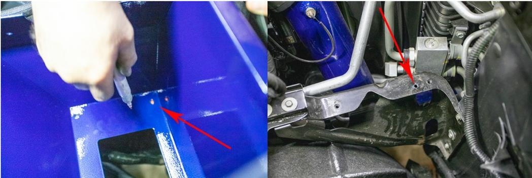
11. Adjust air box position, then use a paint pen to mark location on the lower brace that needs to be drilled for the included nutsert. Remove lower air box and drill marked hole as shown. Verify that nothing is under the location being drilled before making the required hole in the bracket.
