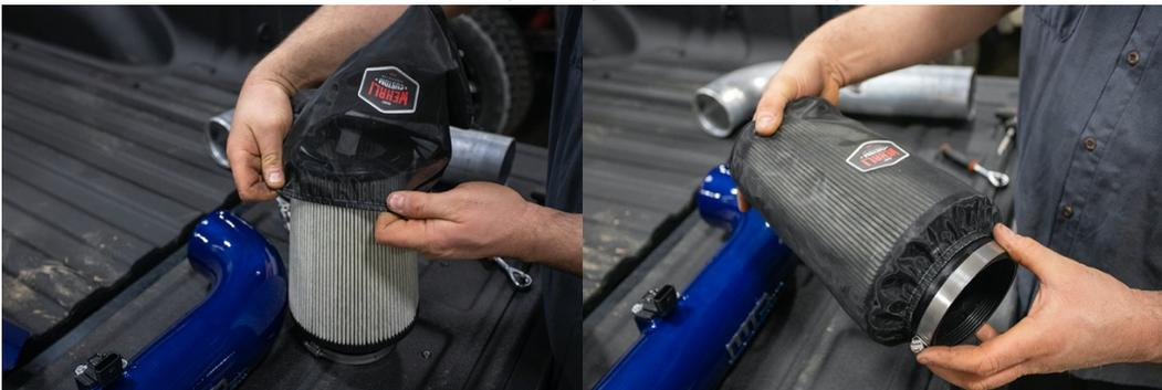
16. Install pre-filter cover and clamp on air filter as shown.
