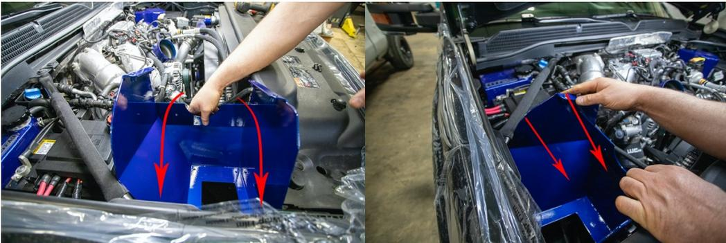
9. Install lower air box as shown. It may be necessary to gently bend rear wall of the box to clear the fender brace if you choose to leave in place as shown. **This box goes in without force.**
