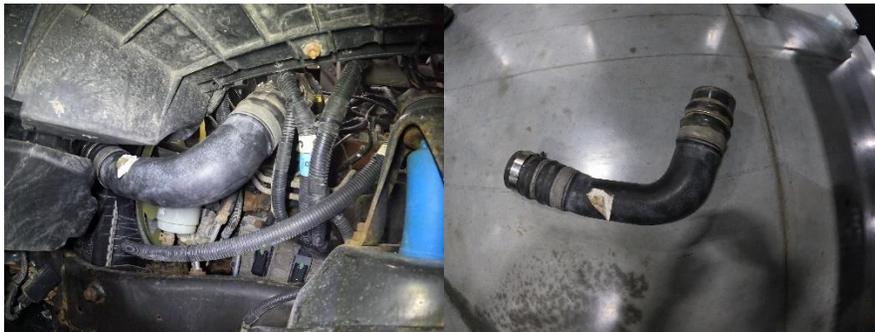
10. Clean the intercooler outlet and install the new boot only tightening the clamp at the intercooler. Install the boot at the intake air valve.
