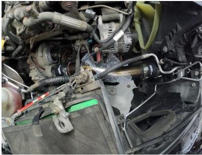
9. Remove the cold side intercooler pipe from the driver side of the engine compartment. This has one clamp at the intercooler outlet and one at the intake air valve.
