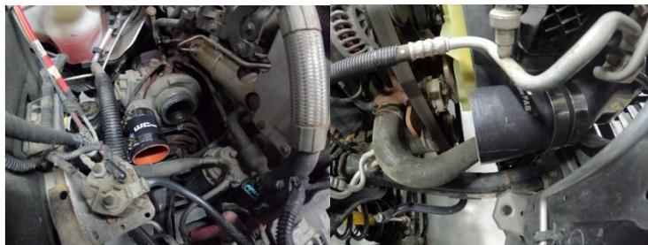
7. Install the intercooler pipe into the boot at the turbo. While holding the pipe in line with the intercooler inlet, you should be able to slide the boot onto the intercooler pipe. Position all clamps and pipe for proper clearance to other objects as shown in picture below.
