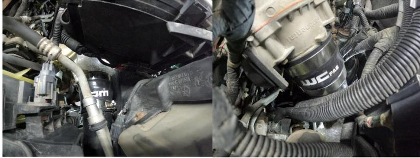
12. It is highly recommended at this point to boost test the system and check for any leaks.
