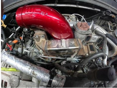
21. Install coolant hose into back side of EGR cooler, then install new EGR gasket from front section to rear section & tighten bolts to **18 LB FT.**
