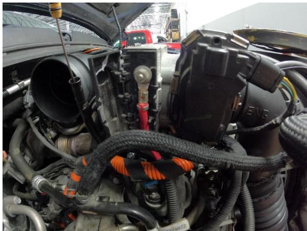
5. Remove the passenger side intercooler pipe connection at the intake air valve by rotating the locking ring at the intake air valve counterclockwise slightly while pulling the pipe towards the front of the truck with a flat head screwdriver for assistance.
