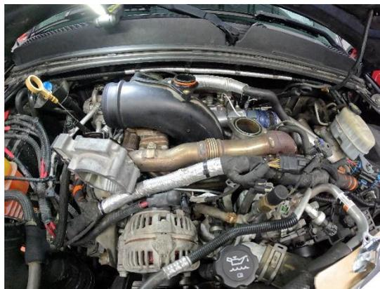
9. Remove grid heater from truck by removing the last 10mm bolt on the bottom left corner.
