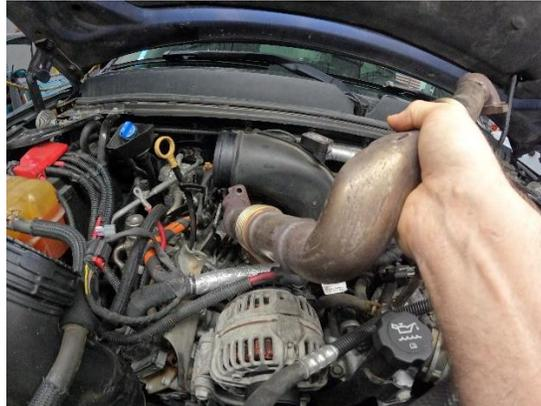
12. Remove two 10mm bolts from PCV to factory intake horn & disconnect connectors attached to bracket.
