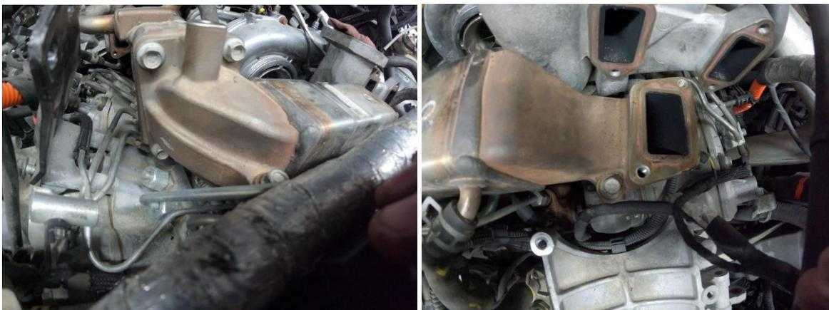
17. Remove hoses from front and rear section of front EGR cooler and remove from truck.
