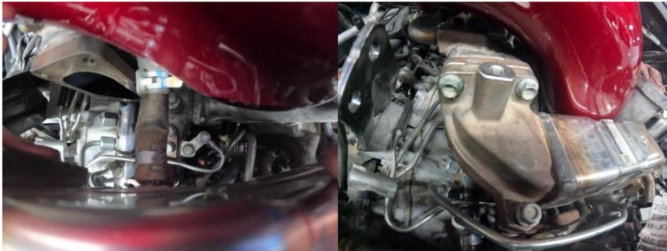
22. Install front EGR mount bolts & torque to **18 LB FT** and reconnect front coolant hose.
