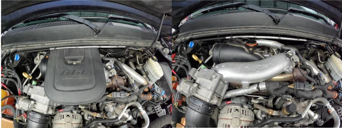
4. Remove the MAP sensor connector, intake air valve connector, grid heater connectors & battery cable from grid heater using a 10 mm socket.
