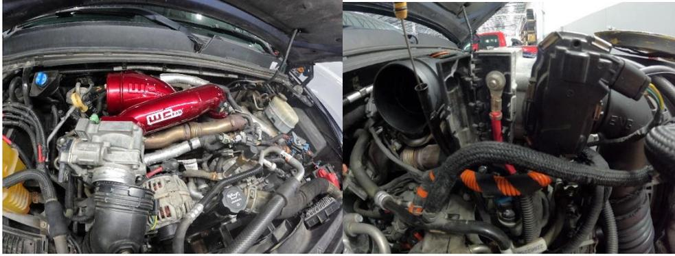
28. Due to size increase of intake horn, the temp sensor bracket for the connectors can be zip tied up to wire harness on firewall or to heater hose, but either way is fine.
