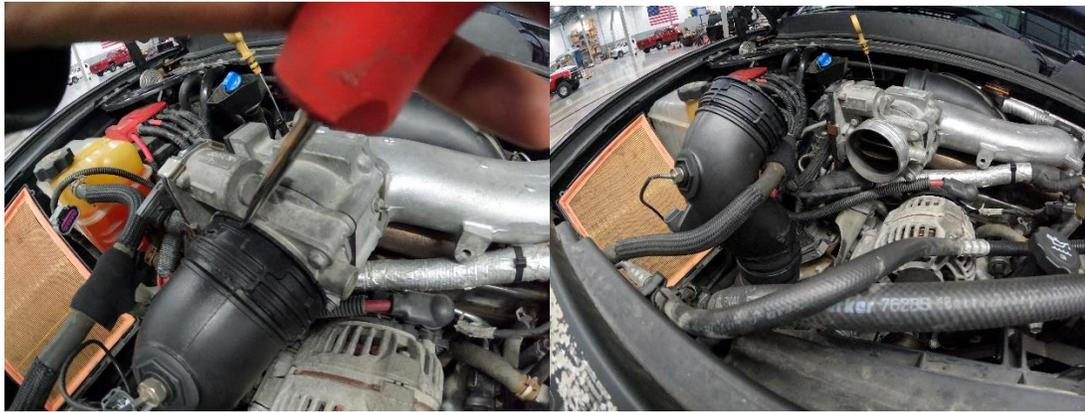
6. Loosen the four 10mm bolts on the intake air valve & remove from the truck.
