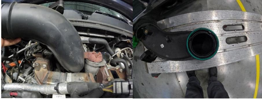
15. Disconnect EGR valve electrical connectors & four 13mm bolts to y-bridge to remove valve.
