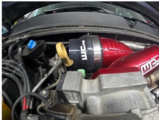
33. Transfer MAF and humidity sensor (if equipped with one) into WCFab Intake Pipe and make sure sensor is closest to the intake horn or it may throw codes due to air flow in wrong direction. If you don't have a humidity sensor, use supplied block off plate.
