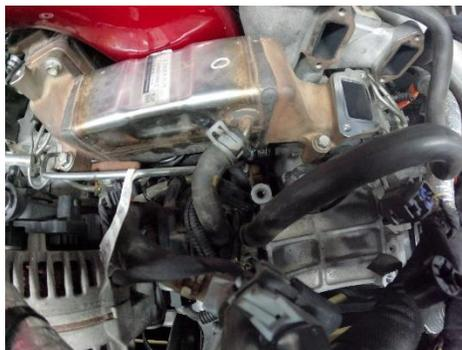
23. Install EGR valve & torque to **18 LB FT**. Verify new gaskets with old gaskets before installing them if unsure of locations to place them.
