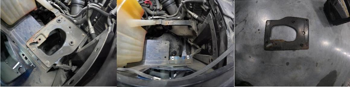
31. Install new air box using factory hardware.
