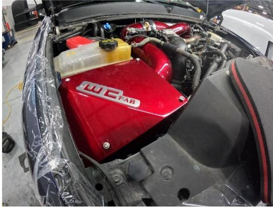
36. Reconnect batteries, start the engine and check for any leaks throughout new piping.
