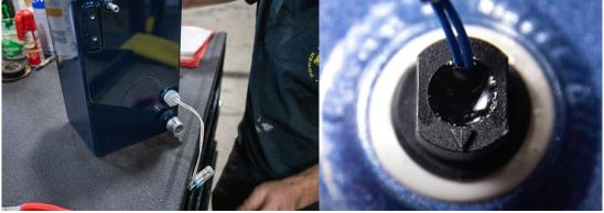
12. When properly installed, the sensor should not have threads showing, just like the picture shown. The arrow on the sensor faces up to make sure the sensor will function. These are pipe threads and need to be tightened all the way to seal up.
