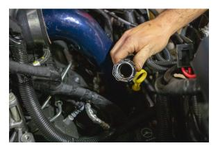
11. Install the level sensor in the new tank using pipe thread sealant. NOTE: White hex sensor needs arrow pointing up, black round sensor needs arrow pointing down.
