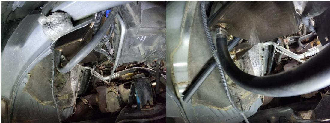
11. Install the overflow hose on the side of the tank facing the engine and position the loose end behind the tank near the firewall as shown.
