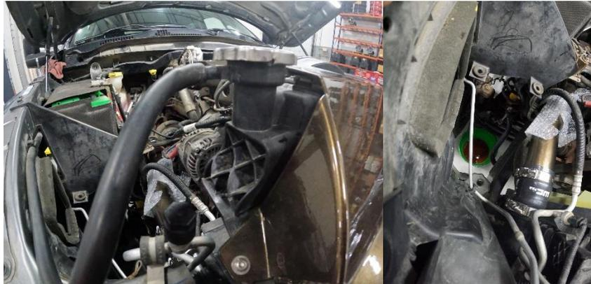
4. Remove the four 10mm nuts holding the tank to the firewall.
