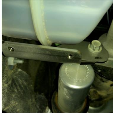
3. Remove the brake reservoir cap. Remove the rubber gasket from the factory cap and transfer it to new billet cap if using (sold separately).
