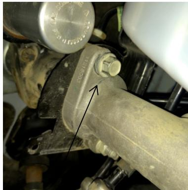
2. Slide the mounting bracket in onto the bolt and tighten. Make sure the mounting point for the reservoir cover is vertically level.
