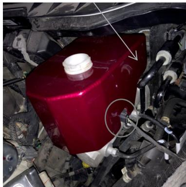
5. Install both Allen head bolts to mount the cover to the mounting bracket.
