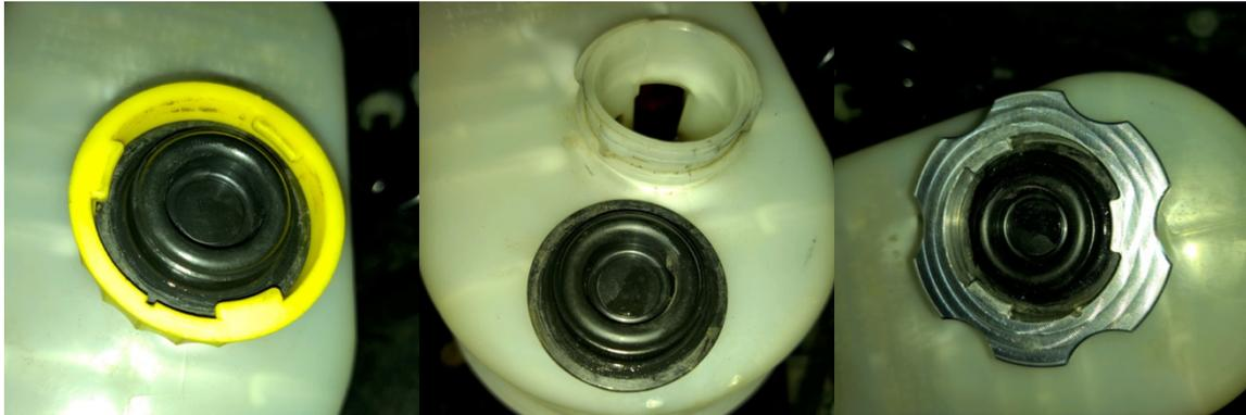
4. Install powder coated cover by slipping in at an angle. Be sure to not break the level sensor (circled in photo). Make sure the cover is on the outside of the mounting bracket that was previously installed in step 2.
