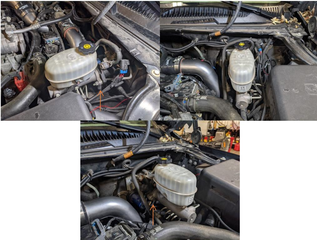
1. Loosen the two 15 mm nuts on the front of the master cylinder. If the stud starts to rotate, hold it on the back side with a wrench while loosening and tightening the nut.
