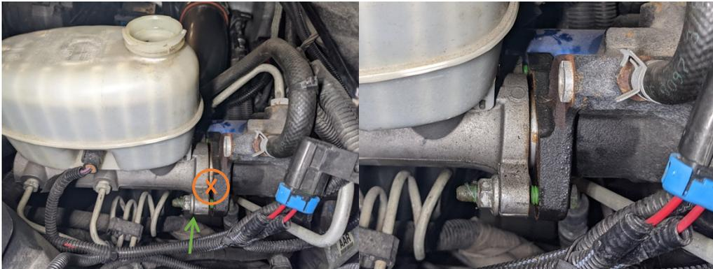
3. Slip the new cover between the nuts and master cylinder. Do not install between master cylinder and hydro boost.
