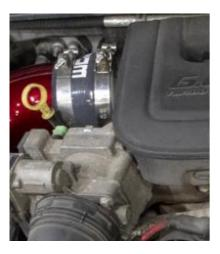
7. Transfer MAF and humidity sensor (if equipped with one) into WCFab Intake Pipe and make sure sensor is closest to the intake horn or it may throw codes due to air flow in wrong direction. If you don't have a humidity sensor, use supplied block off plate.
