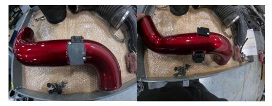
8. Place air filter in box & install pipe into boot first & air filter second before tightening clamps down. Once clamps are tight, plug in the MAF & CAC Temp Sensors.
