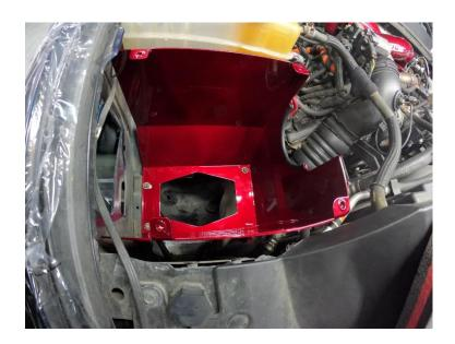
6. Install boot & clamp onto intake horn.
