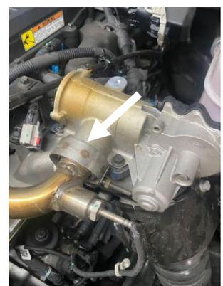
**STEP 3:** Remove the intake horn; Remove the 6 bolts that retain the intake horn to the cylinder head intake shelf. Remove the 1 bolt that retains the dipstick tube to the intake horn. Remove the T-Bolt clamp from the intake tube.
