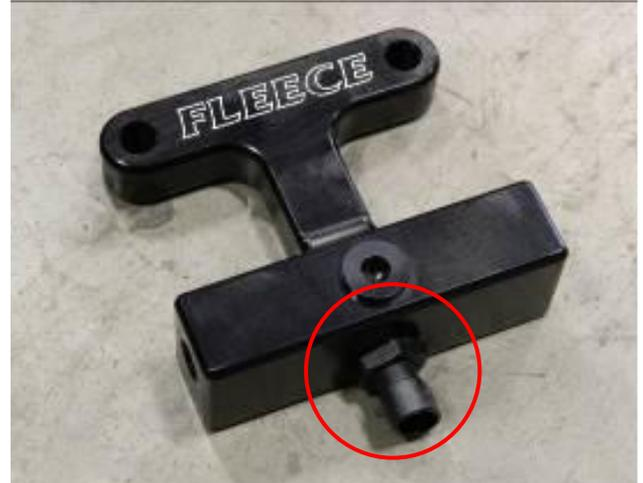
STEP 11: Using the two factory fasteners, install the Fleece Performance Fuel Delete Block to the engine in the same location as factory fuel filter housing.
