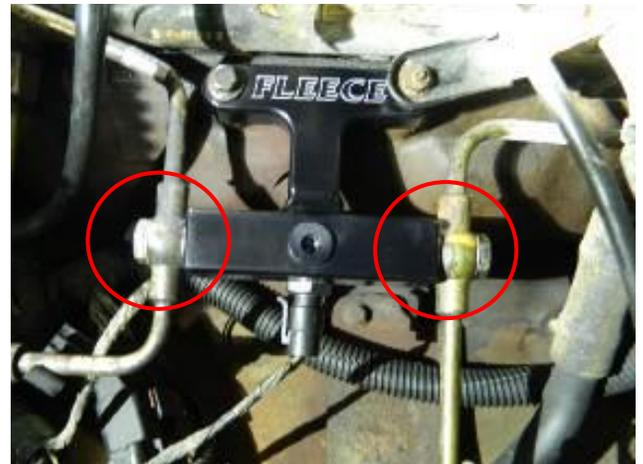
STEP 13: Tighten the fuel filter delete fasteners and torque the banjo bolts to factory spec's.
