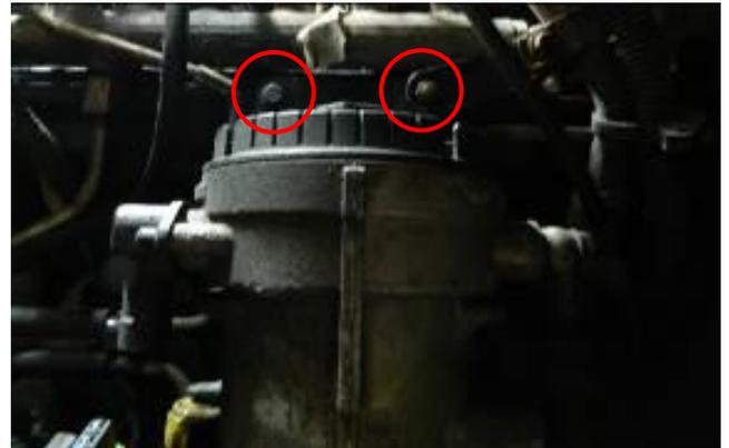
STEP 8: Remove the fuel filter assembly
