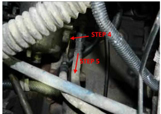
STEP 5: Use a 10mm socket to remove the fuel return line support bracket bolt.
