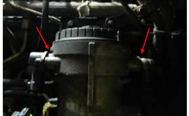
STEP 7: Use a 10mm socket to remove the two fuel filter assembly bolts that secure the assembly to the side of the head.
