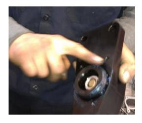
STEP 8: Ensure that the coolant bypass thermostat housing is firmly seated on the back of the engine block and fasten it securely into place using the supplied M12 flange head bolts using a 16mm socket. (item 6).
