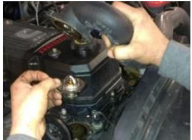
STEP 8: Position the thermostat housing riser block (item 3) on top of thermostat. The O-ring should be facing upward with the threaded fitting facing towards the rear of the vehicle.
