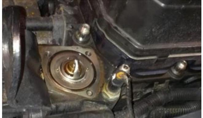
STEP 7: Remove the stock thermostat. Inspect it for wear and proper function. With a Scotch-Brite™ pad and degreasing solution, thoroughly clean the sealing surface of the stock thermostat and thermostat housing. Be sure to remove any foreign debris, and reinstall the OE thermostat.
