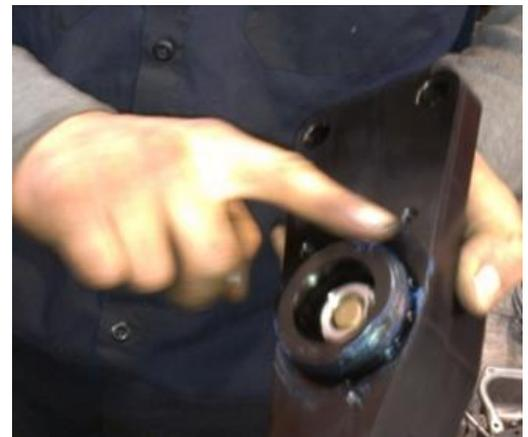
STEP 14: Ensure that the coolant bypass thermostat housing is firmly seated on the back of the engine block and fasten it securely into place using the supplied M12 flange head bolts using a 16mm socket. (item 7).
