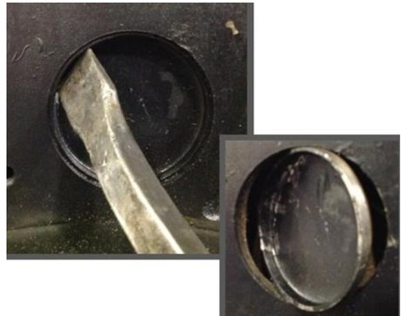
STEP 11: With the freeze plug removed, using a Scotch-Brite™ pad and a degreasing solution, thoroughly clean the block surface area from the head down to the rear cover, as well as the bore where the freeze plug was previously installed. Be sure to remove any dirt or foreign debris.
