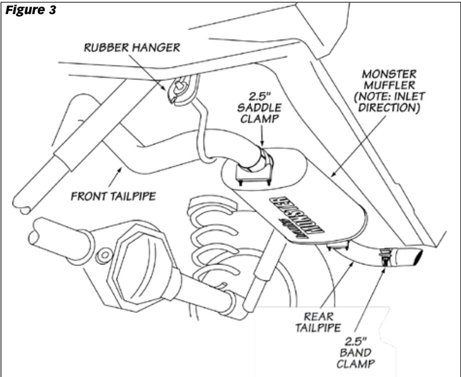
and flat under rear bumper. Loosely tighten the 2.5" clamp.
