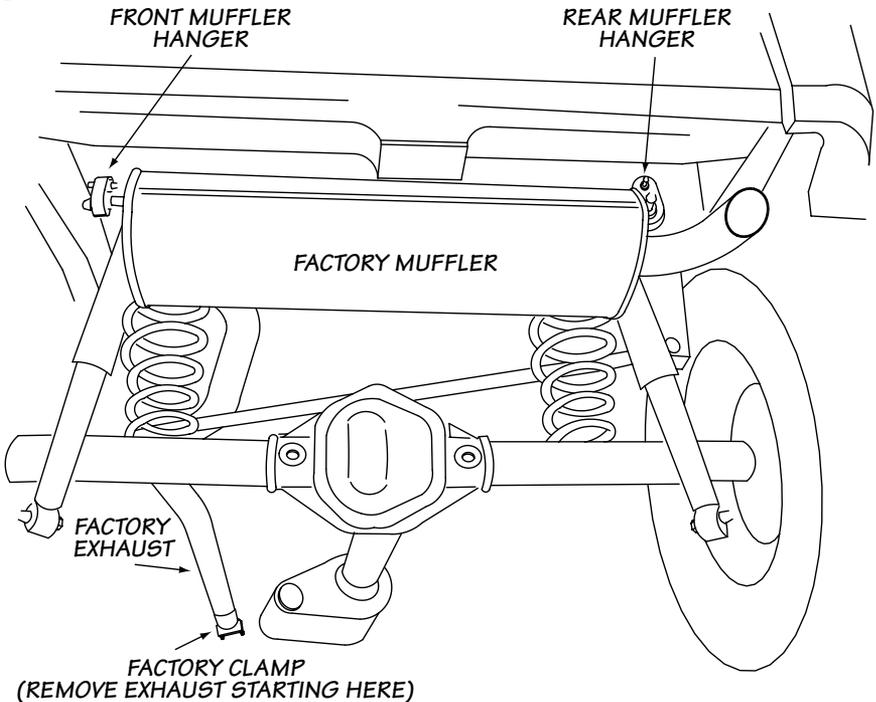
hanger pin into the vehicle's rubber hanger. Loosely tighten the 2.5" clamp.
