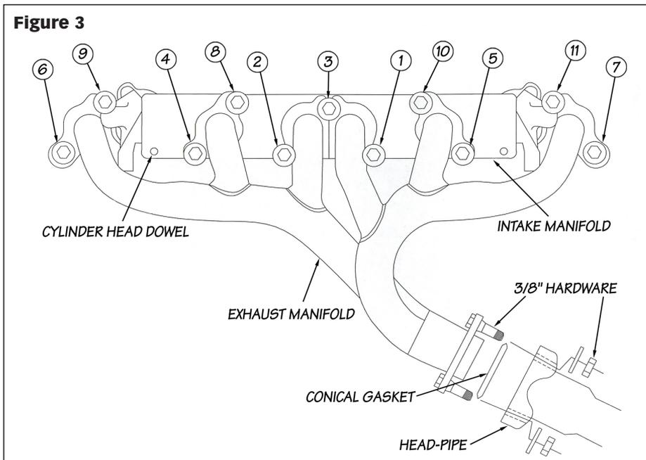
**13.** Install bolts 1, 2, 4 and 5 about three turns into engine block. Guide the intake manifold onto the cylinder head dowels. Loosely install all remaining intake/exhaust factory bolts. Be sure Banks TorqueTubes and intake manifold seats flush as bolts are tightened.
