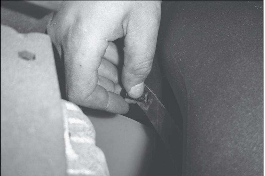
**17.** Locate the supplied MAF to intake tube hose (Item 6) with the square notch cutout and the MAF sensor attached to Banks Ram-Air filter cover. Slide the MAF to intake tube hose onto the MAF sensor. Make sure the square notch cutout and the tab on the MAF sensor line up and fit snug. Tighten the hose clamp (Item 2) to secure the MAF to intake tube hose to the MAF sensor but leave the hose clamp on the other end of the hose adapter loose. See **Figure 14**.
