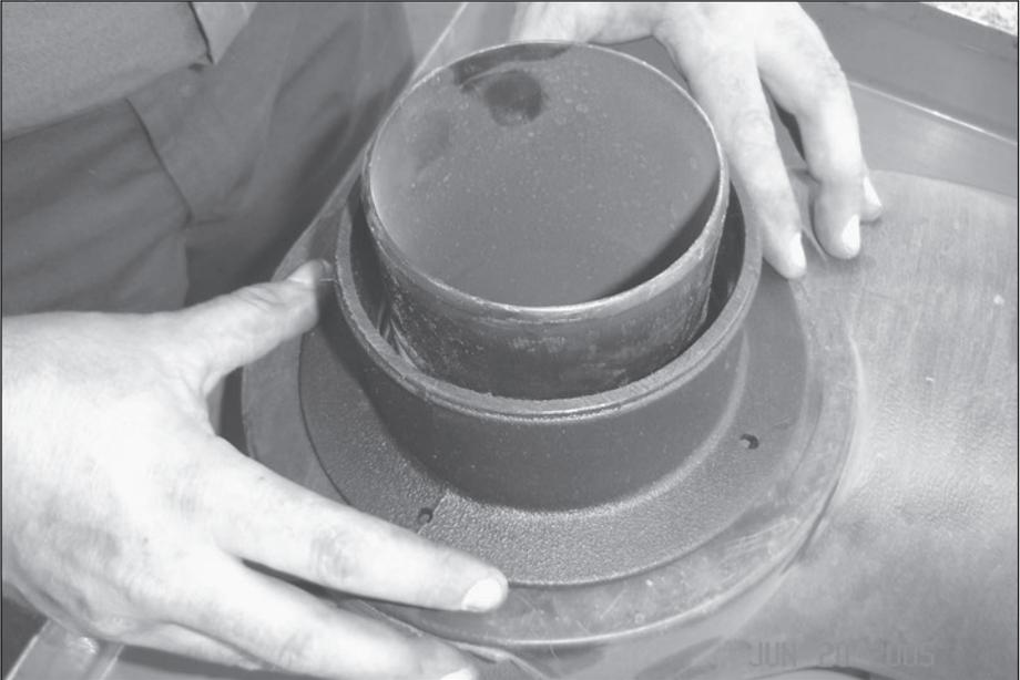
**22.** Visually center the Banks snorkel outlet adapter over the stock snorkel outlet. Using the Banks snorkel outlet adapter as a template, drill a  $\frac{3}{16}$ " hole into the snorkel through one of the existing holes in the adapter. See **Figure 18**.
