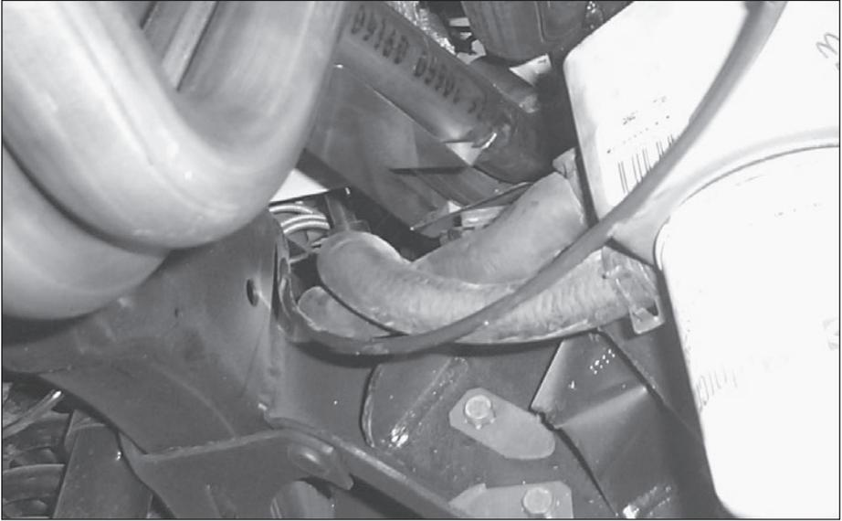
**20.** Make sure the O-ring is on the dipstick tube, and reinstall it into the hole in the engine block. Reattach the dipstick tube bracket to the cylinder head with the factory hardware.
