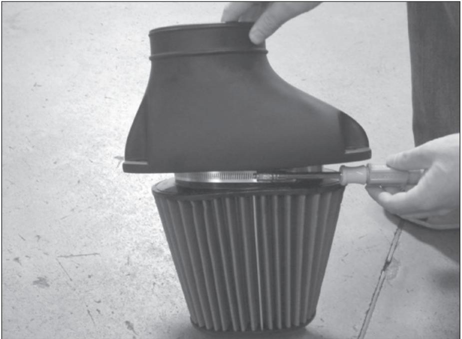
**20.** Locate the Banks filter cover. Install the Banks filter onto the Banks filter cover. Tighten Banks filter hose clamp. See **Figure 12**.
