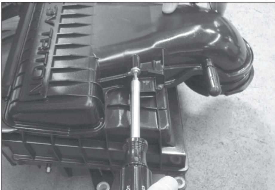
**9.** Using the supplied screws, lightly tighten the MAF sensor to the Banks High-Ram intake tube.
