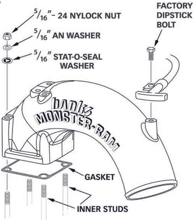
Monster-Ram in place on the studs. Twist a Stat-o-seal washer over the inner two studs, then over each stud install a flat 5/16" AN washer. Install a 5/16" - 24 nylock nut on each stud and tighten all four evenly between 11-12.5 ft-lb (140 to 150 Inch Pounds) See **Figure 5**.
