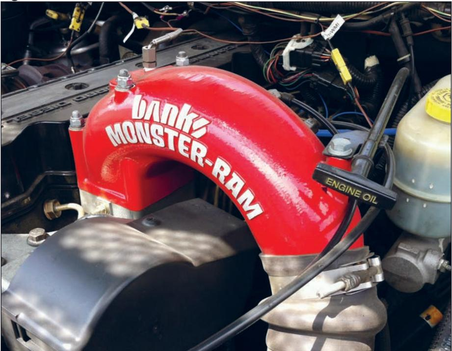
**18.** Remove all rags from the intercooler up-pipe opening and reconnect the rubber hose from the intercooler up-pipe to the Monster-Ram and tighten the clamp to 100 Inch Pounds.
