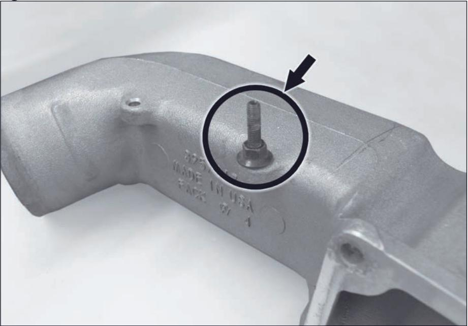
gouge the mating surfaces of the parts, completely remove the stock gaskets from both sides of the heater element block and intake manifold, using a gasket scraper as needed. Clean and dry all sealing surfaces thoroughly.
