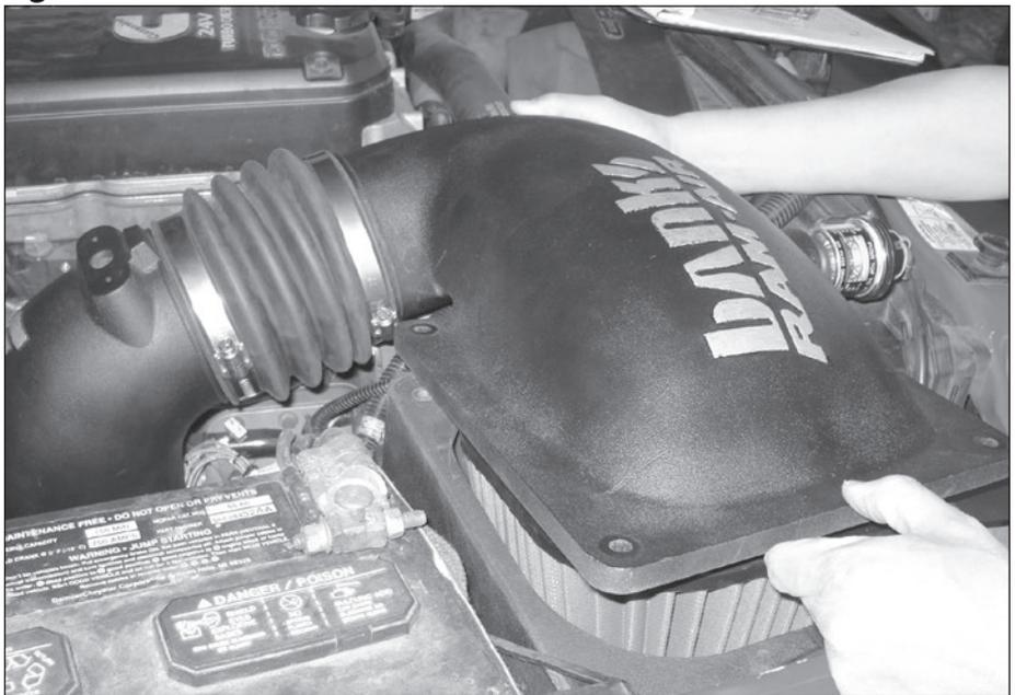
**27.** Install Banks air filter onto the Banks cover. Note the audible snap. Tighten the hose clamp on the air filter. Make sure the air filter is lined up with the alignment groove. See **Figure 15**.
