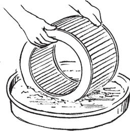
**NOTICE:** NEVER use gasoline, steam, caustic solutions, strong detergents, high-pressure nozzles, or cleaning solvents to clean the filter element. All of these can cause harm to the filter media as well as SHRINK and HARDEN the rubber end caps.
