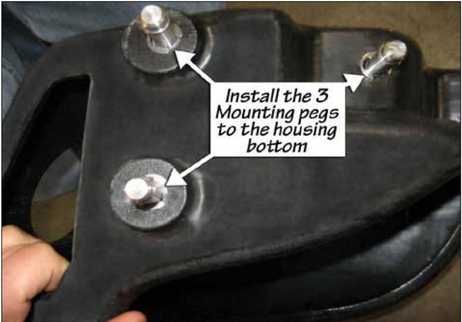
**7.** Remove the air filter housing (bottom) by lifting up from the passenger side of the engine compartment and set aside. See **Figure 4**.
