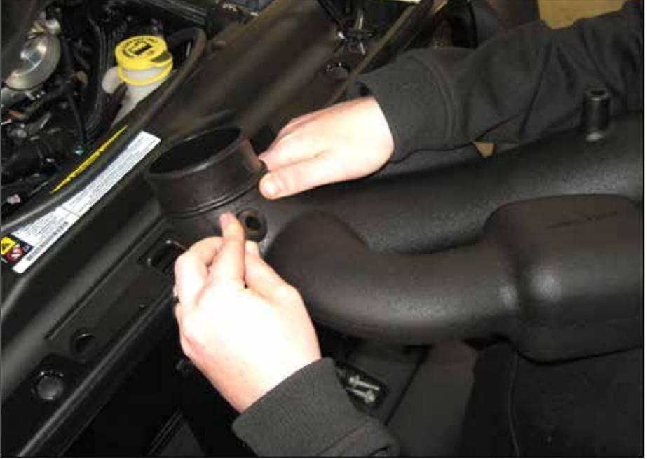
**Figure 7- Connecting air filter with intake tube**
