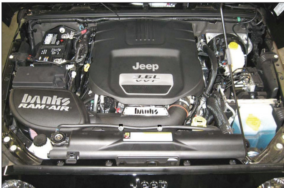
Figure 8- Installed Banks Ram-Air Intake System
