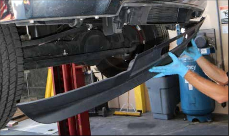
**1.** On the 2013-up Ram 2500 and 3500, the Intercooler is located behind the front bumper, underneath the radiator. To begin, remove the front bumper air dam. This requires removing the two bolts and 15 retainer clips that attach the air dam to the bumper. These can be accessed from the back of the bumper. This requires a 10mm wrench or socket and a body clip removal tool. **Figure 1**
