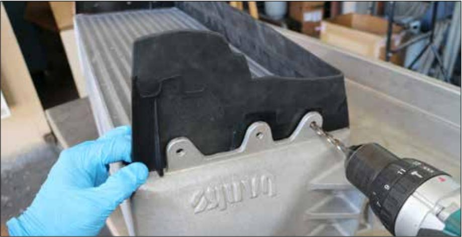
**9.** Place the front air intake shroud for the intercooler on your new Banks Techni-Cooler. Mark and drill the sides of the shroud using a 1/4-inch drill bit so you have three mounting holes on each side. Take care not to drill these holes too big, as the push pins that mount the shroud require a tight fit in the hole to be secure. Do not attach the front shroud to the intercooler at this time. **Figure 9**
