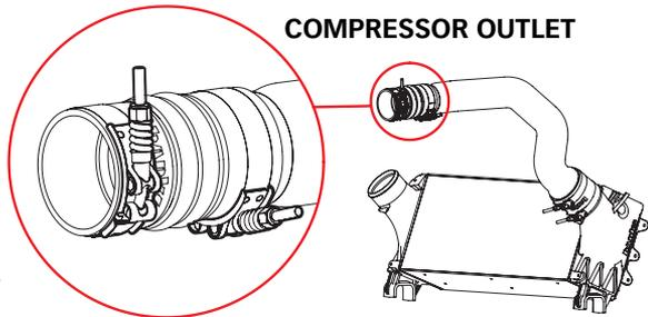
**Figure 11c** Clamp Assembly Positions
