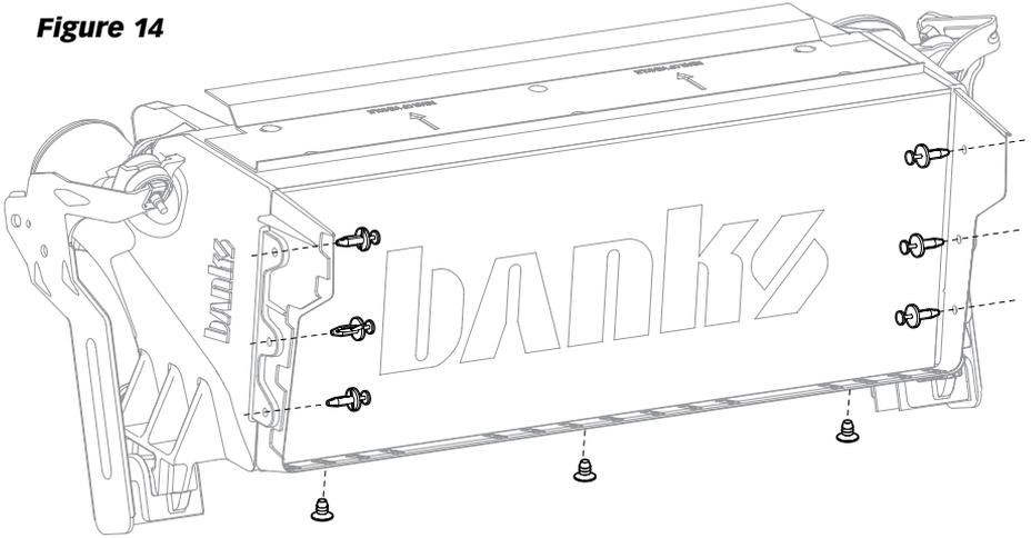
**15.** Install the trimmed front air intake shroud onto your Banks Techni-Cooler, using the six supplied push pins, and ratchet fasteners. **Figure 14**
