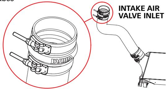
**Figure 11b** Clamp Assembly Positions
