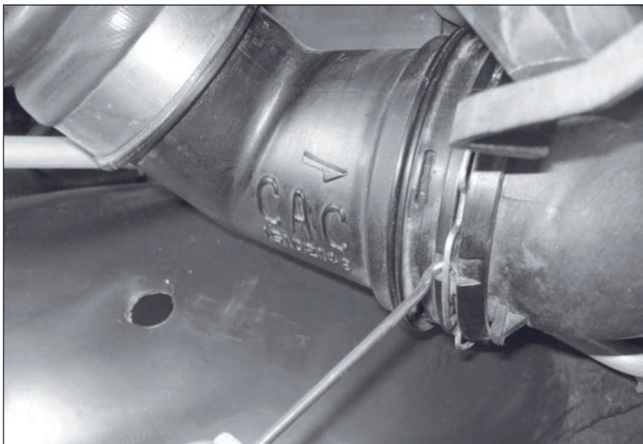
**Figure 18** Passenger side boost tube
