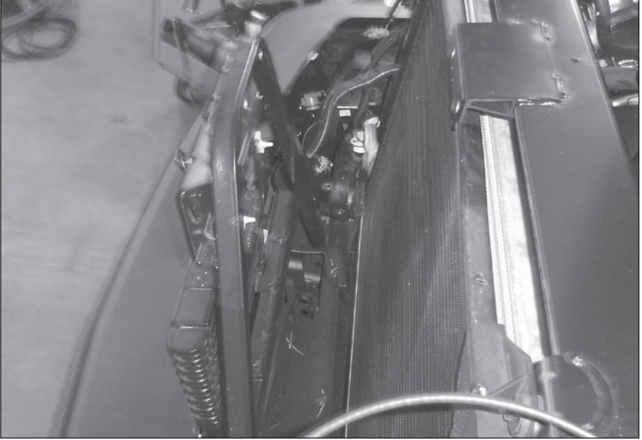
**Figure 7:** Upper Charge Air Cooler (CAC) attachment bolt
