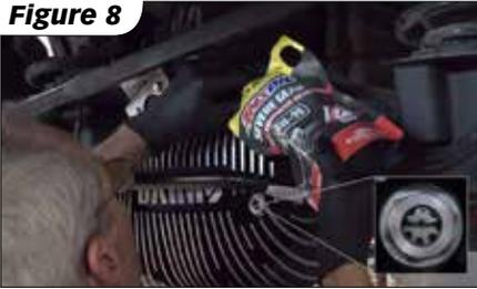
**11.** Install the fill plug using a 3/8" square drive.
