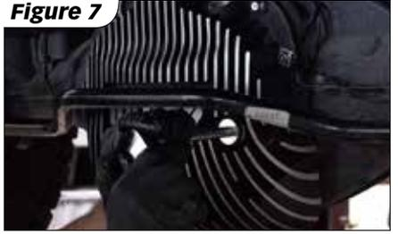
**8.** Install the drain plug(s) using a 3/8" square drive.
