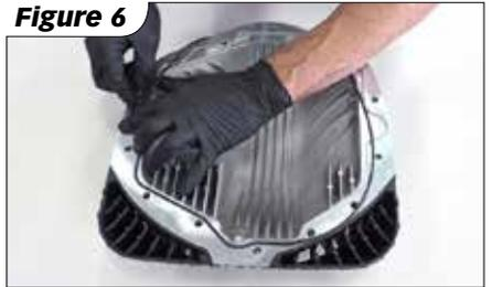
**7.** Install the Banks cover and re-attach brackets to the cover using included M8 bolts. Apply small amount of threadlocker on the bolts. Torque the bolts to 12 lb/ft (29 N.m) using a 10mm 12 pt socket.
