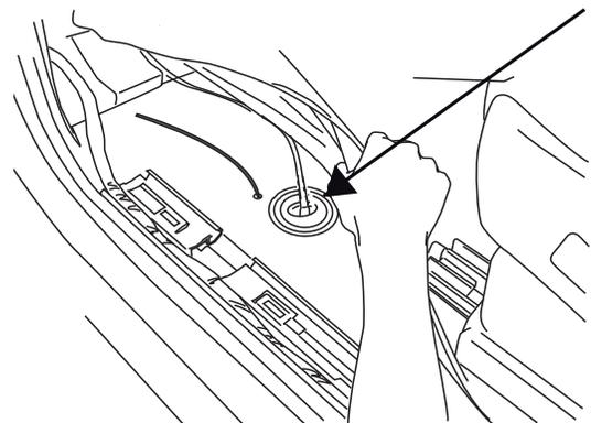
**On the Driver side, Do Not zip tie the Wire Harness to the Brake Lines.**
