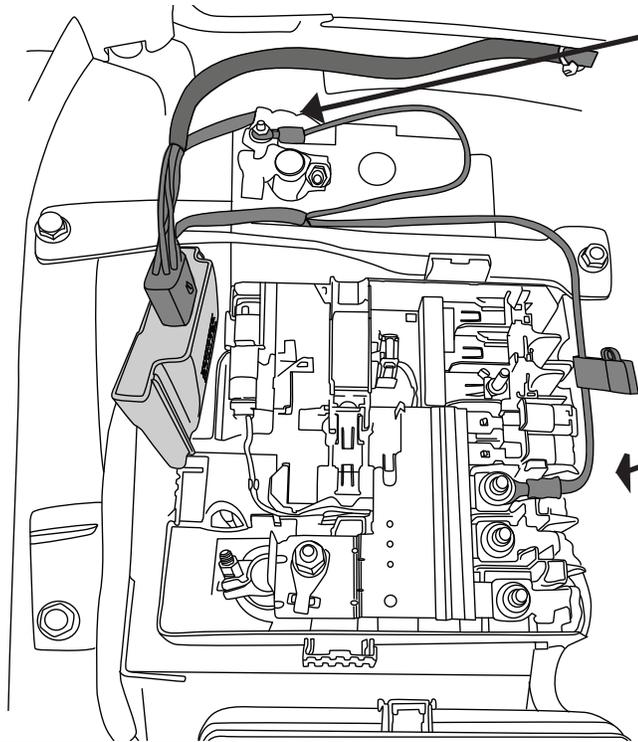
Battery terminal accessory stud, install under factory nut.
