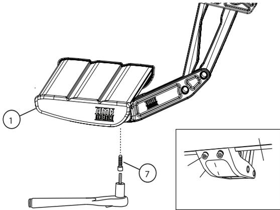
On each side of the vehicle measure from the rear linkage to end of the board. Measurement should be approximately 11" as shown below.
