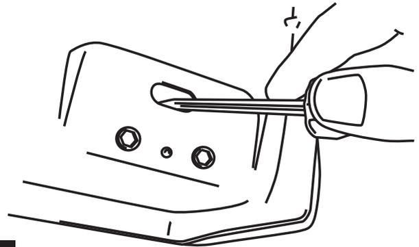
**11** NOTE: Hold Rivet tool with wrench while loosening bolt.
