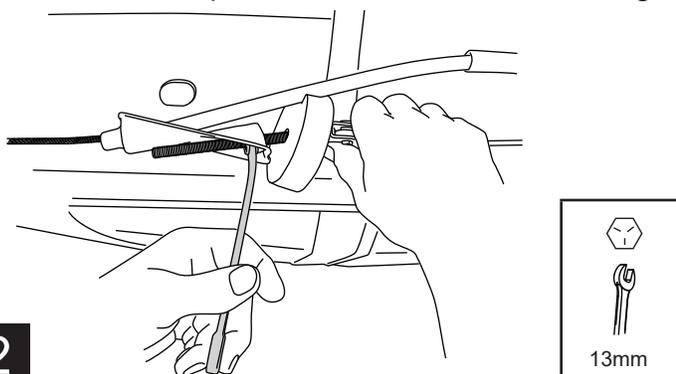
After gaining enough slack, detach brake cable as shown below. This detachment point is located just to the rear of the adjustment nut.
