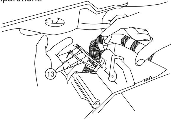
Insert controller into tie-wrap loops and cinch down securely. The tie-wraps should cinch down into channels on controller surface.
