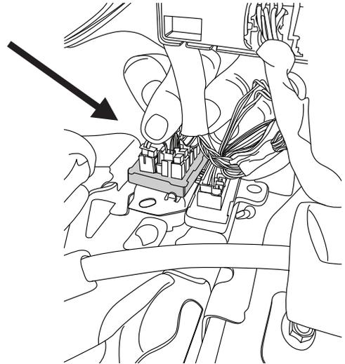
**Note: It's best to reach from both sides when installing 2 pin plug. Any open port on green plug can be used.**
