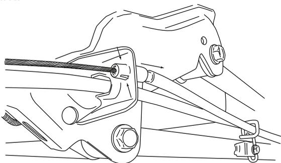
Attach brake cable guide to supplied Brake Cable Bracket (27) and mount bracket with supplied hardware (24,25,26) . Reattach brake cable and readjust brake cable adjustment nut to original position.
