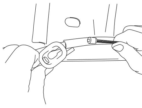
Remove brake cable guide from frame by depressing locking tabs and sliding guide out through hole. Unthread brake cable from frame mount.
