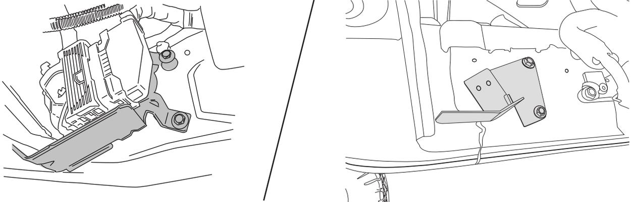
While holding brake cable adjustment nut with wrench (located on driverside along frame, towards the rear), loosen brake cable to allow for slack. Mark position of nut before loosening.
