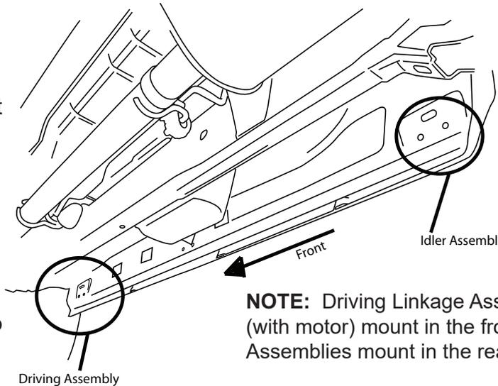
**NOTE:** Driving Linkage Assemblies (with motor) mount in the front; Idler Assemblies mount in the rear.
