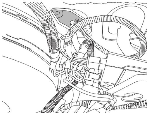
Tape leading end of wires together and push through rubber boot to cabin side of the firewall. Silicon lubricant may be used for ease of passage. The trigger wires will come out just above and to the left of the brake pedal.
