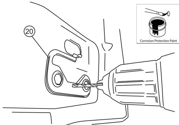
Once hole is drilled insert a piece of string or wire through hole in Reinforcement Plate. Set plate into position.
