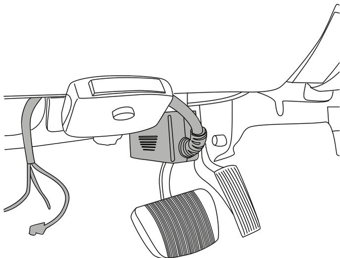
Locate side access cover of dash and remove to gain better access to 2 pin plug for OBD harness installation.
