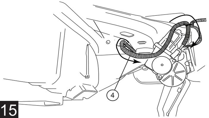
On each side of the vehicle measure approx. 7" back from front linkage and 8" forward of the rear linkage. Pre drill using an 1/8" drill bit and final drill to 9/32" thru pinch weld at marked locations. Insert grommet into drilled holes. Insert lamp wires through the grommets. (Silicon lube will help wires slip through grommets.) Affix lamp to rocker panel surface. Make sure lamp is affixed to a flat, clean surface.
