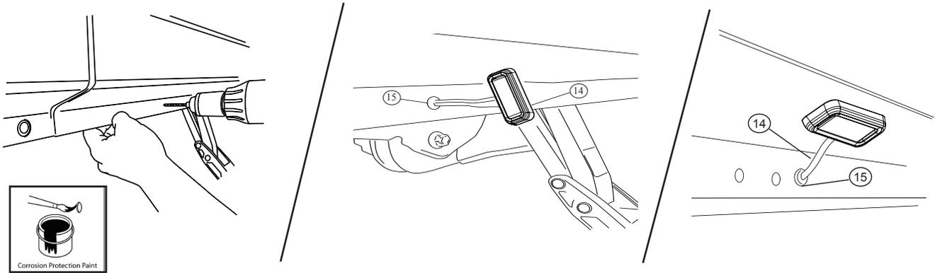
Using supplied butt connectors (13) connect the lamp wires. Red to Red, Black to Black. Once Crimped use heat gun to shrink tube. Close and wrap conduit with electrical tape. Secure all loose wires with cable ties. Pull lamp wires upward to avoid any wire snagging.
