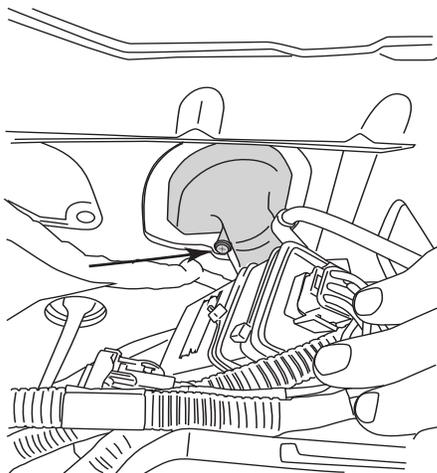
Tape leading end of wires together and push through rubber boot to cabin side of the firewall. Silicon lubricant may be used for ease of passage. The trigger wires will come out just above and to the left of the brake pedal.
