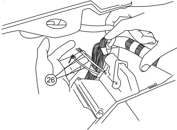
Insert controller into tie-wrap loops and cinch down securely. The tie-wraps should cinch down into channels on controller surface.
