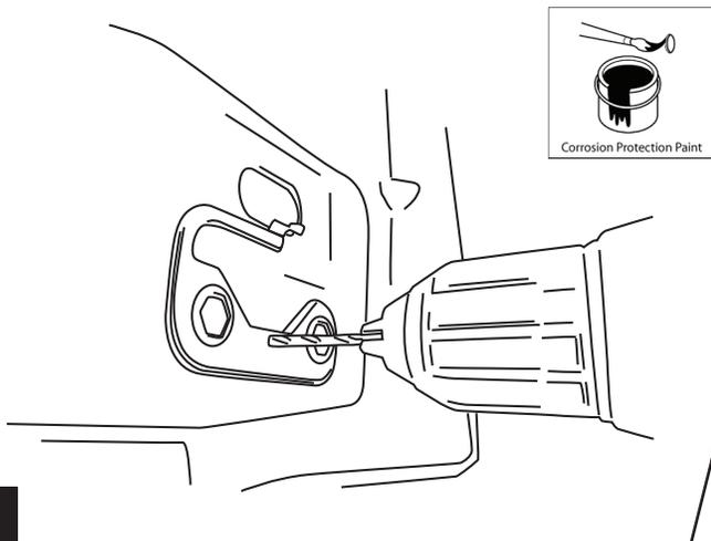
Once hole is drilled insert a piece of string or wire through hole in Reinforcement Plate. Set plate into position.
