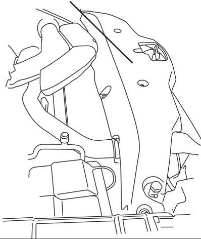
Mount controller with the two 11" tie wraps to factory conduit. Route wire harness under core support and down toward controller. Attach harness to controller (make sure connector locking tabs fully engage).
