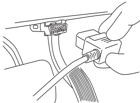
**OBD II install:** Use Supplied Posi-Lock™ connectors to attach the Plug and Play Module to the Harness. Attach matching colors on the harness to the wires on the module. Plug in module to OBD II port on the vehicle. Secure harness with supplied tie wraps. **Note: If the OBD II pass thru harness (76404-01A) was purchased see install sheet supplied in packaging. The pass through harness allows for an open port for other accessories. See below for a brief description.**
