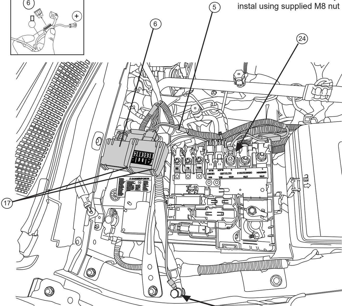
Negative terminal accessory stud to attach black wire.
