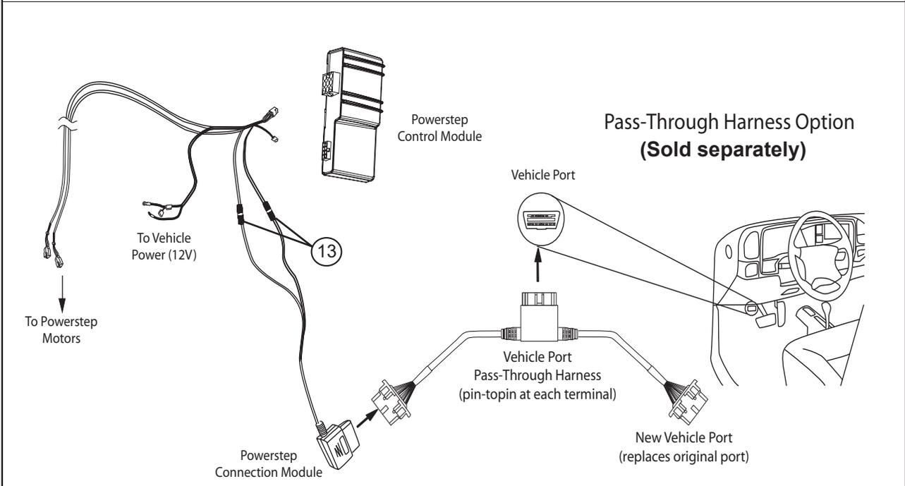
Plug in module to OBD port on the vehicle.
